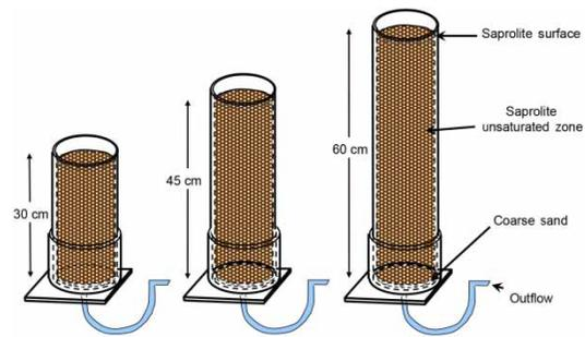
**Figure 2** | A replicate set of saporlite-filled cylinders with saporlite in lengths of 30, 45, and 60 cm.
