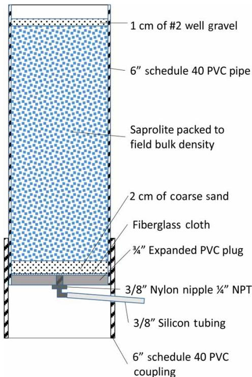
**Figure 1** | Cross-section of a saporlite-filled cylinder showing how it was constructed (1" = 2.54 cm; NPT: American National Standard Pipe Thread).
