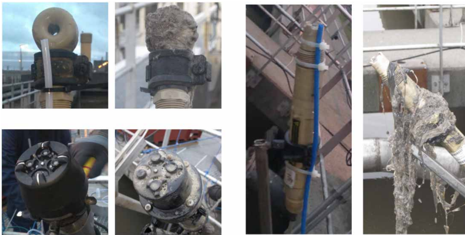
Figure 2 | Sensors in their ideal condition versus their typical operating condition. Top-left: conductivity; bottom-left: \text{NH}_4\text{-N} , K and pH; right: pH (Vanrolleghem 2014).
