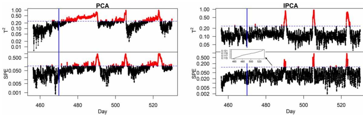
**Figure 3** | Fault detection results of PCA and IPCA for normal operation (dashed blue line: 99% confidence limit; solid vertical blue line: onset of the fault). The small plot in the IPCA chart shows the adaptive threshold for SPE. Please refer to the online version of this paper to see this figure in color: <http://dx.doi.org/10.2166/wst.2020.368>.
