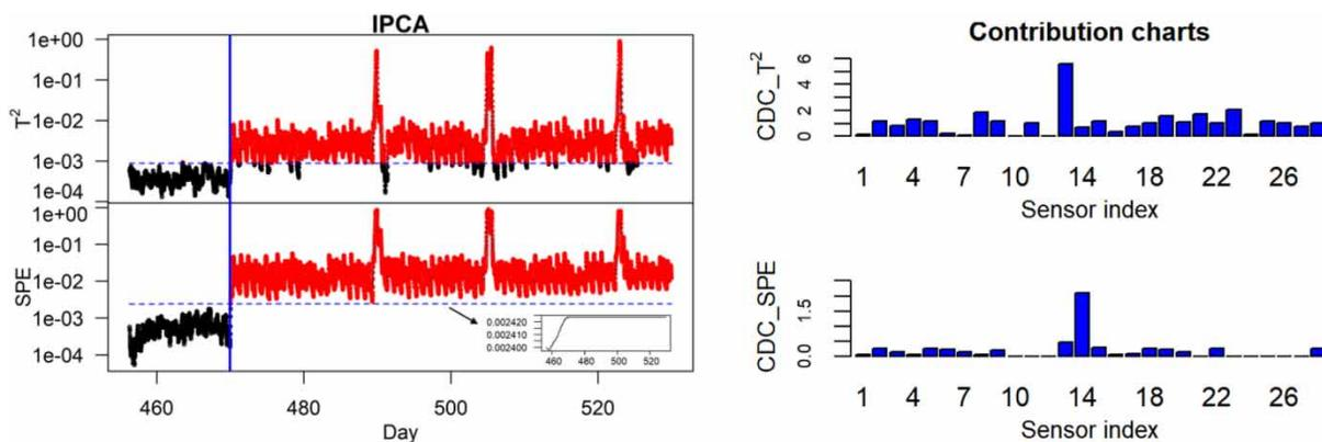
**Figure 6** | Fault detection and diagnosis results of IPCA for a step-change in the settling velocity of the secondary clarifier (dashed blue line: 99% confidence limit; solid vertical blue line: onset of the fault). The small plot inside the IPCA chart shows the adaptive threshold for SPE. Please refer to the online version of this paper to see this figure in color: <http://dx.doi.org/10.2166/wst.2020.368>.
