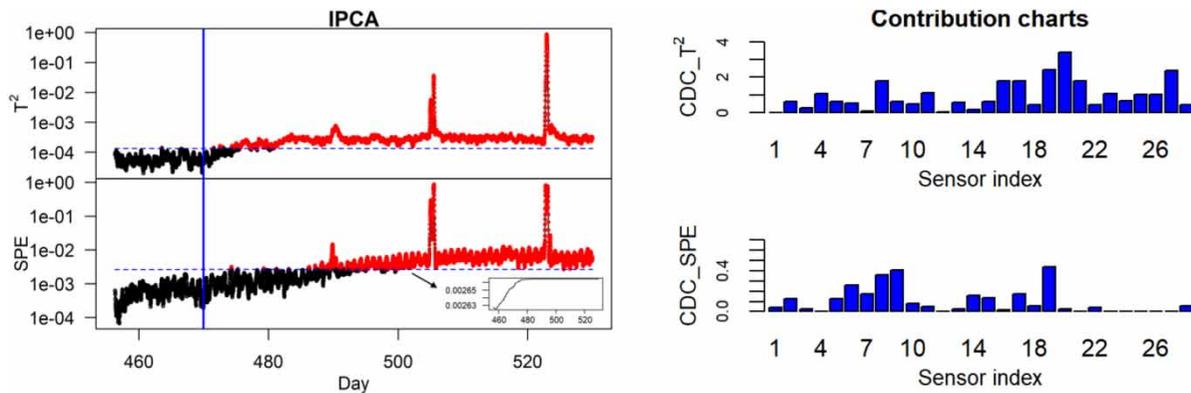
**Figure 5** | Fault detection and diagnosis results of IPCA for a step change in AD inorganic nitrogen (dashed blue dashed: 99% confidence limit; solid vertical blue line: onset of the fault). The small plot inside the IPCA chart shows the adaptive threshold for SPE. Please refer to the online version of this paper to see this figure in color: <http://dx.doi.org/10.2166/wst.2020.368>.
