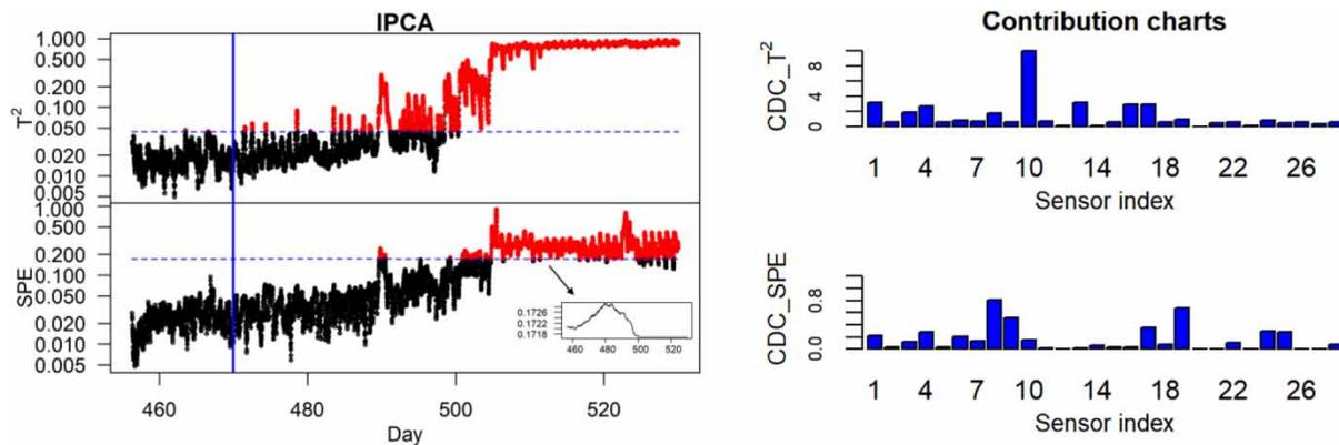
**Figure 7** | Fault detection and diagnosis results of IPCA for a step change in the specific growth rate of the autotrophs (dashed blue line: 99% confidence limit; solid vertical blue line: onset of the fault). The small plot inside the IPCA chart shows the adaptive threshold for SPE. Please refer to the online version of this paper to see this figure in color: <http://dx.doi.org/10.2166/wst.2020.368>.
