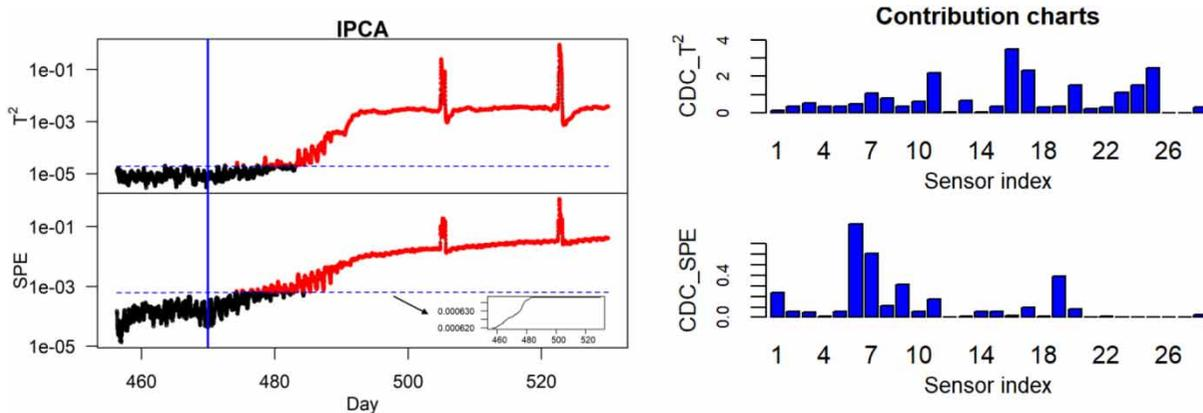
**Figure 4** | Fault detection and diagnosis results of IPCA for drift fault in the dissolved oxygen sensor (dashed blue line: 99% confidence limit; solid vertical blue line: onset of the fault). The small plot inside the IPCA chart shows the adaptive threshold for SPE. Please refer to the online version of this paper to see this figure in color: <http://dx.doi.org/10.2166/wst.2020.368>.
