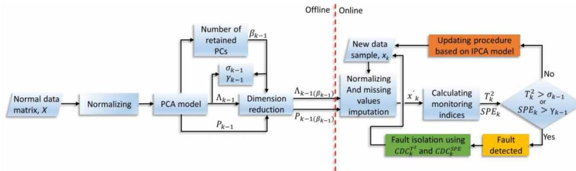
Figure 1 | Adaptive IPCA monitoring diagram.
