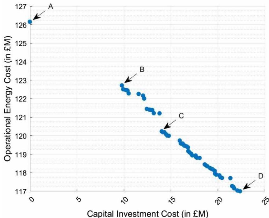
**Figure 3** | Multi-objective trade-off between CAPEX and OPEX costs. Solution A represents no capital investment; Solutions B and D are the lowest and highest combination of capital investment respectively; and solution C is the Pareto efficient solution. There is a gap between solution A and B because the capital investment at solution B is the minimum amount needed to reach an optimal combination of capital investment and operational energy costs.
