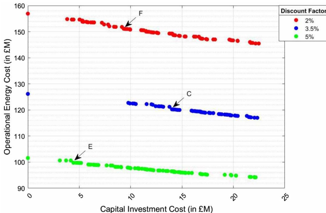
**Figure 5** | Multi-objective trade-off between CAPEX and OPEX costs with different discount rates. Solutions E and F represent higher and lower discount rates respectively. Solution C remains as the original Pareto efficient solution in Figure 3.
