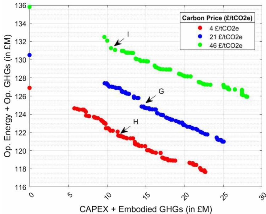
**Figure 7** | Comparison of CAPEX and embodied capital GHGs with operational energy and GHG costs. Solution G is the original pareto efficient solution in Figure 6 which includes the cost of GHGs; Solutions H and I represent higher and lower carbon prices respectively.
