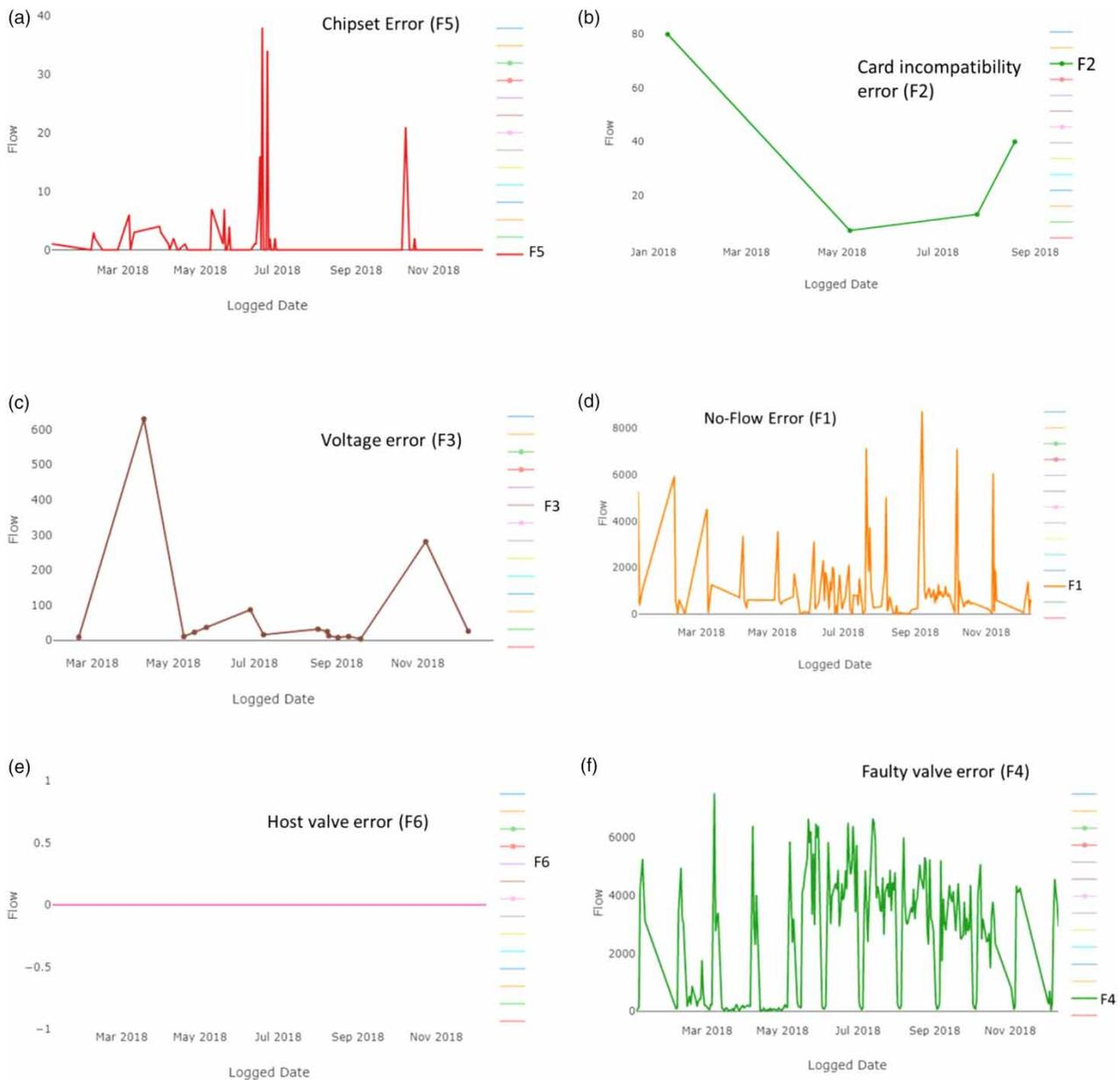
**Figure 4** | Predicted errors/failures on some of the e-taps.
