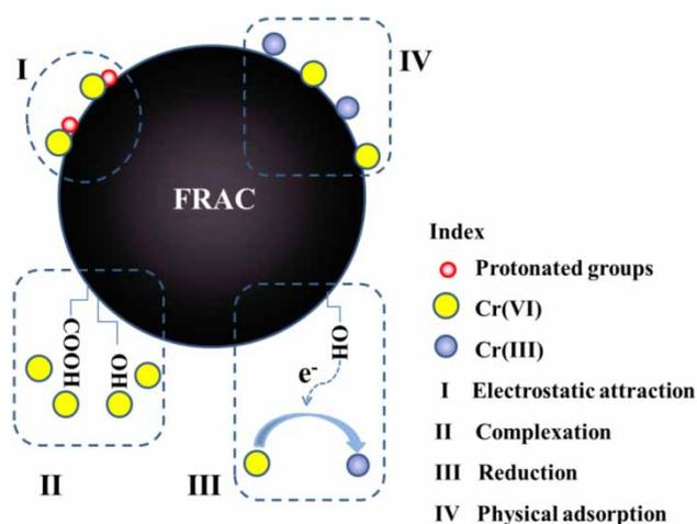
Figure 9 | Adsorption mechanism of Cr(VI) by FRAC.
