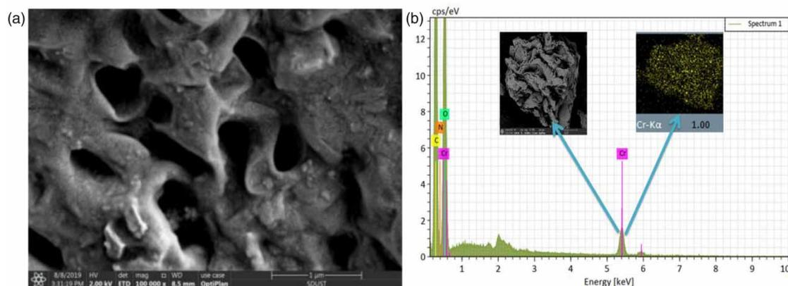
**Figure 4** | SEM of FRAC before Cr(VI) adsorption (a) and SEM, EDS, and Cr mapping of Cr-loaded FRAC (b).
