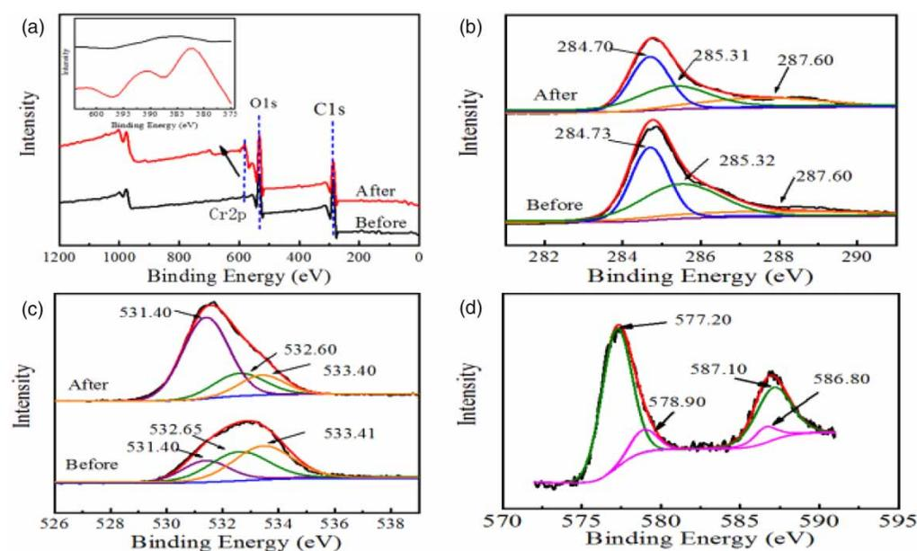
**Figure 5** | XPS survey spectra of FRAC before and after Cr adsorption (a), high resolution XPS spectra of C 1s (b), O 1s (c), and Cr 2p after Cr adsorption (d).
