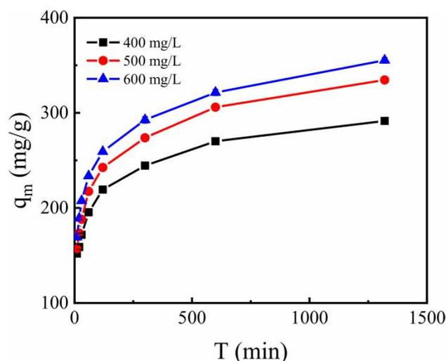
Figure 7 | Effect of contact time on adsorption of Cr(VI) at different initial concentrations.
