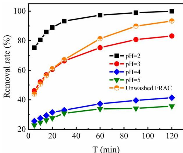
Figure 6 | Effect of pH on adsorption properties of FRAC.
