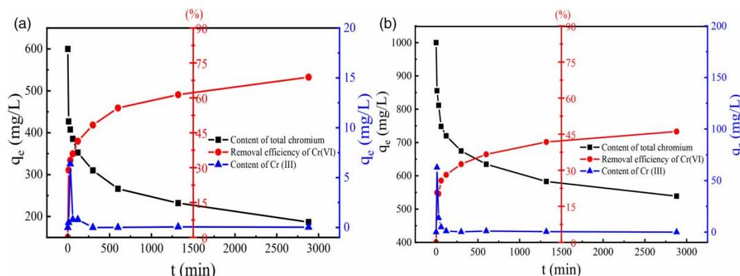
**Figure 8** | The variation tendency of total Cr, Cr(VI) and Cr(III) in solution at different initial Cr(VI) concentrations (a: 600 mg/L; b: 1,000 mg/L).
