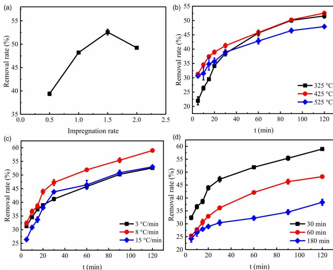
**Figure 1** | Effect of AC preparation conditions on Cr(VI) removal rate: (a) impregnation ratio; (b) carbonization temperature; (c) heating rate; (d) carbonization time (adsorption experiment: initial Cr(VI) concentration; 50 mg/L; temperature, 35 °C; adsorption time, 120 min).
