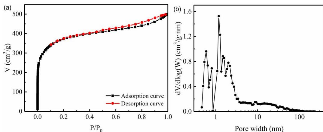
**Figure 2** |  $N_2$  adsorption-desorption isotherms (a) and pore size distribution curve (b) of the obtained FRAC.
