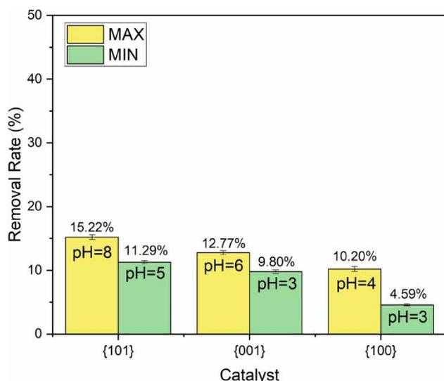
**Figure 8** | The adsorption experiments for ROX (Time = 240 min, C<sub>ROX</sub> = 10 mg/L and C<sub>TiO<sub>2</sub></sub> = 500 mg/L).
