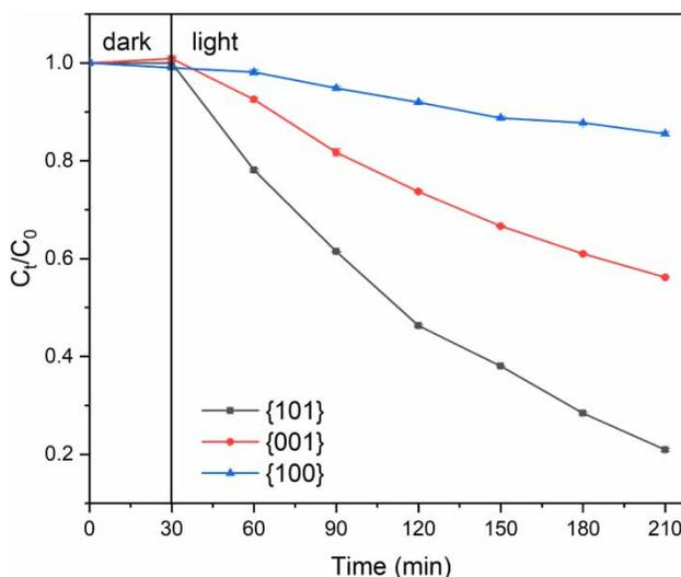
**Figure 1** | Variation of ROX concentration before and during Xenon lamp for three types of TiO<sub>2</sub> at pH 7 (The initial ROX is 100 mg/L and TiO<sub>2</sub> is 2.0 g/L).
