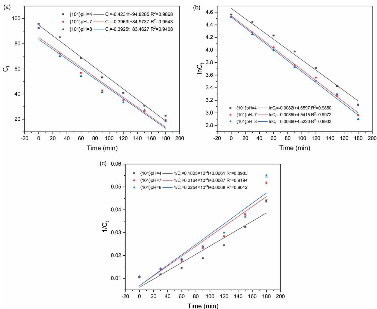
**Figure 3** | Zero-order, first-order and second-order kinetics for photocatalytic oxidation on {101} facet TiO<sub>2</sub> at pH 4, pH 7 and pH 8 ((a) is for zero-order kinetics, (b) is for first-order kinetics, (c) is for second-order kinetics. The initial ROX is 100 mg/L and TiO<sub>2</sub> is 2.0 g/L).
