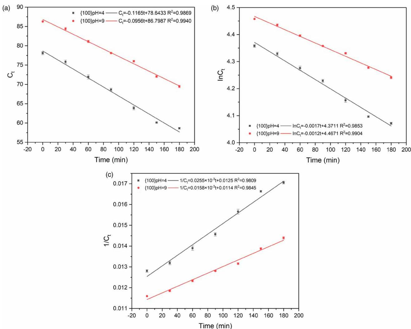
**Figure 5** | Zero-order, first-order and second-order kinetics for photocatalytic oxidation on {100} facet TiO<sub>2</sub> at pH 4 and pH 9 ((a) is for zero-order kinetics, (b) is for first-order kinetics, (c) is for second-order kinetics. The initial ROX is 100 mg/L and TiO<sub>2</sub> is 2.0 g/L).
