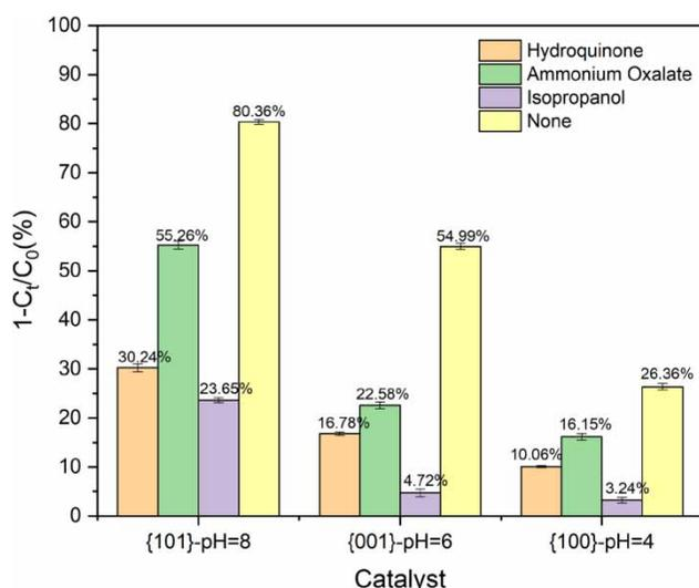
**Figure 7** | Removal rate of ROX ((1-C<sub>t</sub>/C<sub>0</sub>) %) with and without three types of traps. (C<sub>TiO<sub>2</sub></sub> = 2,000 mg/L, C<sub>ROX</sub> = 100 mg/L, C<sub>hydroquinone</sub> = 0.1 mmol/L (or C<sub>ammonium oxalate</sub> = 0.1 mmol/L or C<sub>isopropanol</sub> = 0.1 mmol/L), pH = 8 for {101} facet TiO<sub>2</sub>, pH = 6 for {001} facet TiO<sub>2</sub>, and pH = 4 for {100} facet TiO<sub>2</sub>, and the reaction time is 3 hours as in Figure 2).
