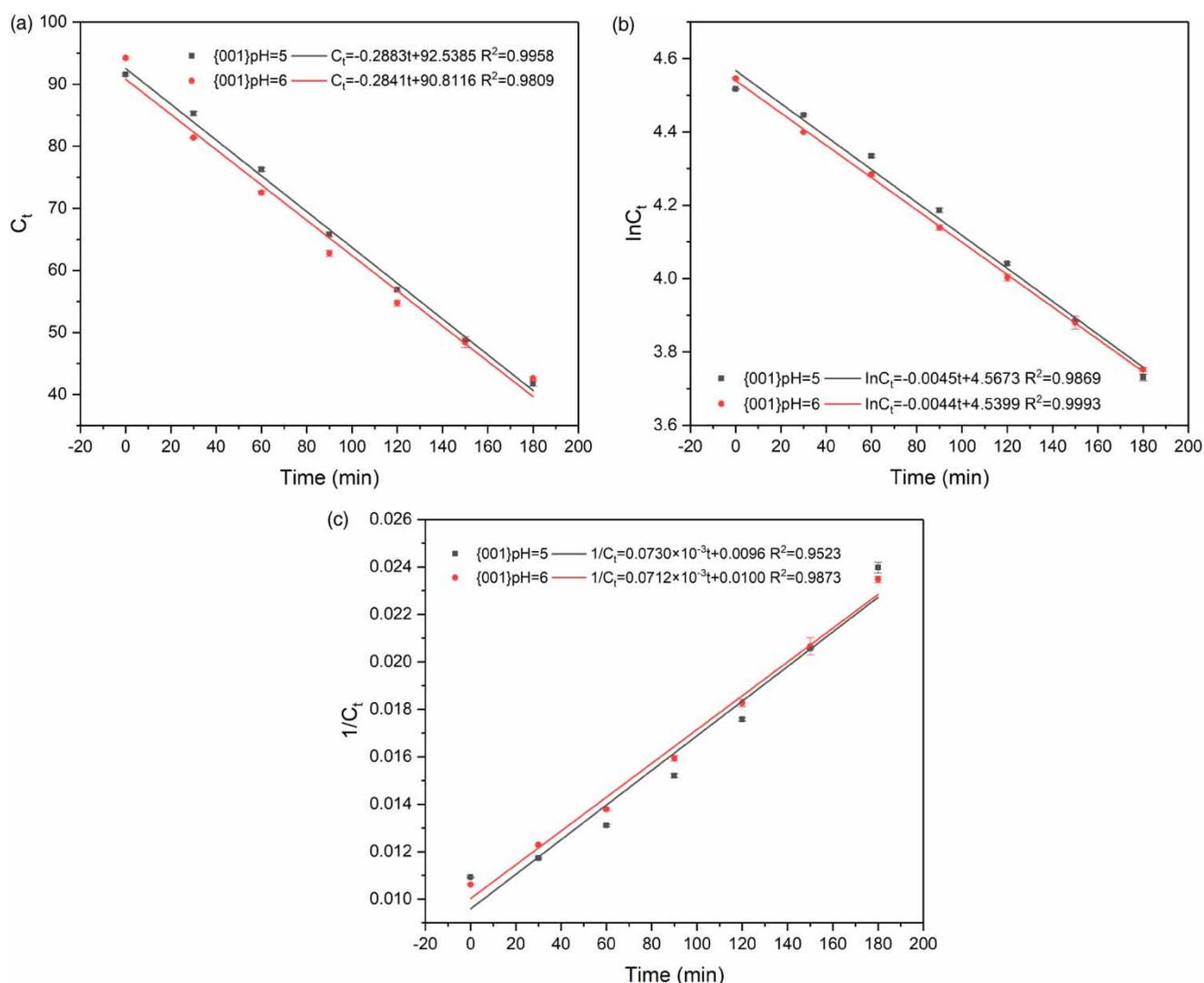
**Figure 4** | Zero-order, first-order and second-order kinetics for photocatalytic oxidation on {001} facet TiO<sub>2</sub> at pH 5 and pH 6 ((a) is for zero-order kinetics, (b) is for first-order kinetics, (c) is for second-order kinetics. The initial ROX is 100 mg/L and TiO<sub>2</sub> is 2.0 g/L).
