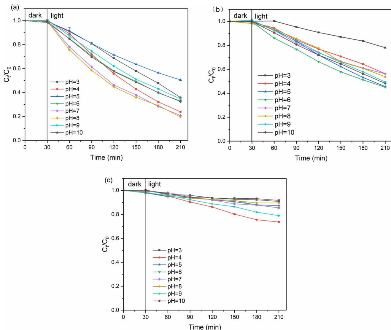
**Figure 2** | Photocatalytic oxidation of ROX at different pH values for three types of TiO<sub>2</sub> (a) is for {101} facet, (b) is for {001} facet, (c) is for {100} facet. The initial ROX is 100 mg/L and TiO<sub>2</sub> is 2.0 g/L.
