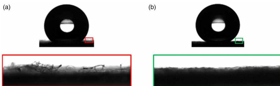
**Figure 3** | Close-up images of (a) neat membrane, (b) coated membrane.
