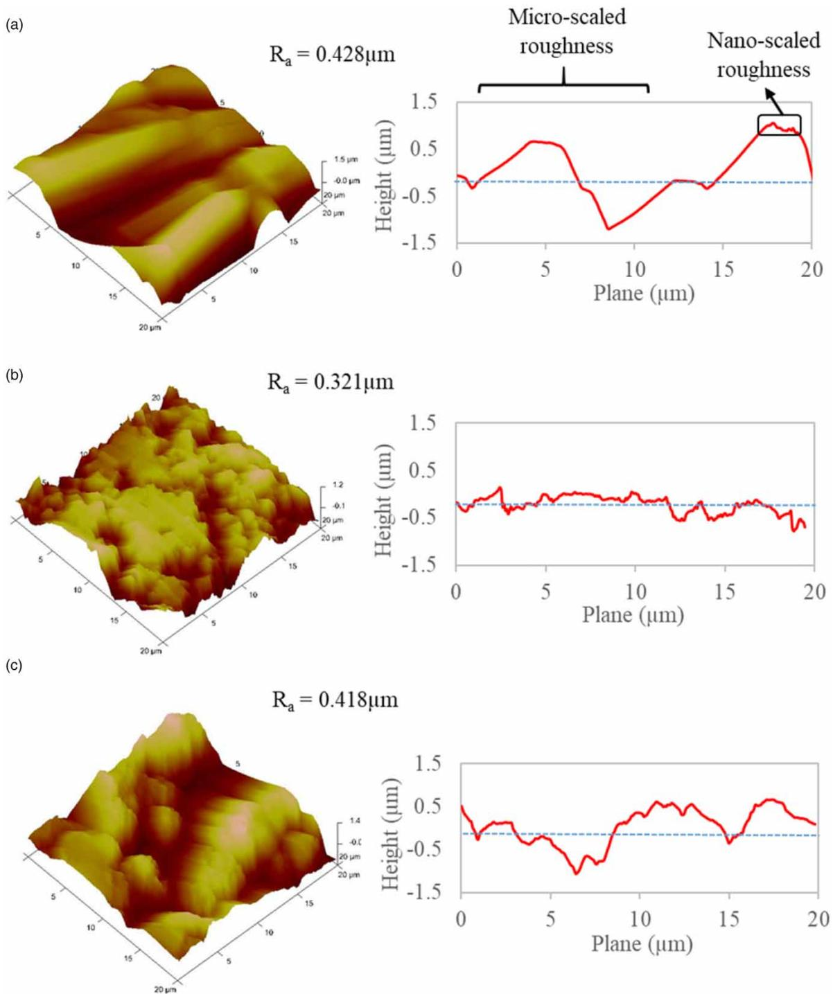
**Figure 2** | AFM analyses of (a) neat PP, (b) PP/6331-L1 and (c) PP/6331-L3 membranes.
