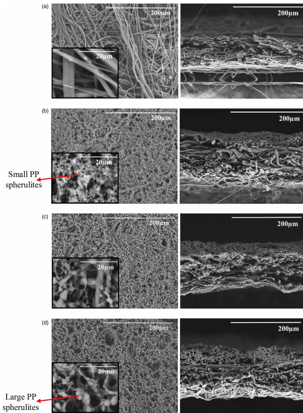
**Figure 1** | SEM micrograph of surface (left images) and cross-sectional (right images) of (a) neat PP, (b) PP/6331-L1, (c) PP/6331-L2 and (d) PP/6331-L3 membranes.
