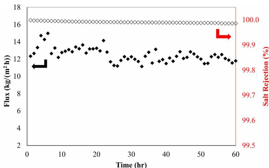
Figure 5 | Flux and salt rejection of PP/6331-L1 in 60 hr long term DCMD performance test.
