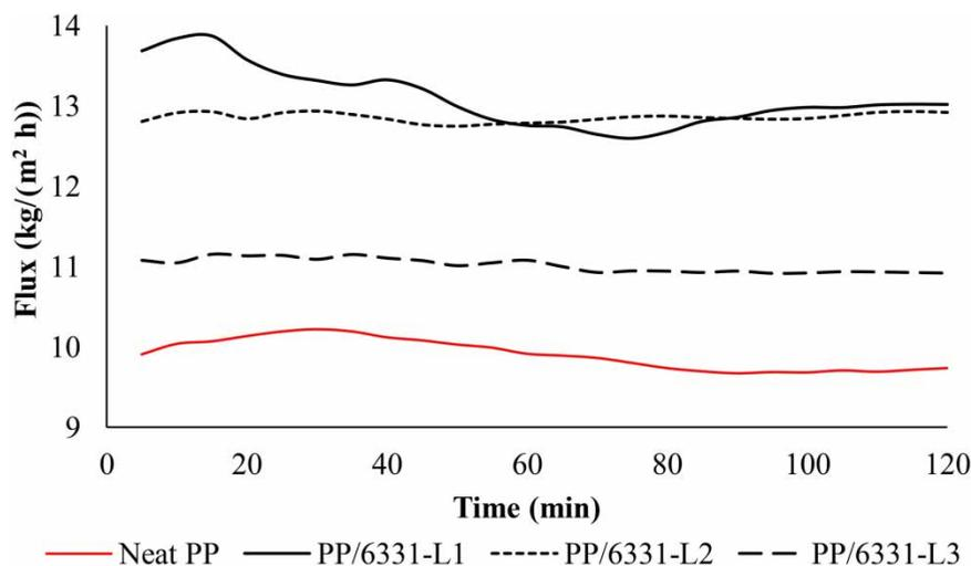
Figure 4 | Flux of neat and surface modified membranes in 2 hr DCMD performance test.
