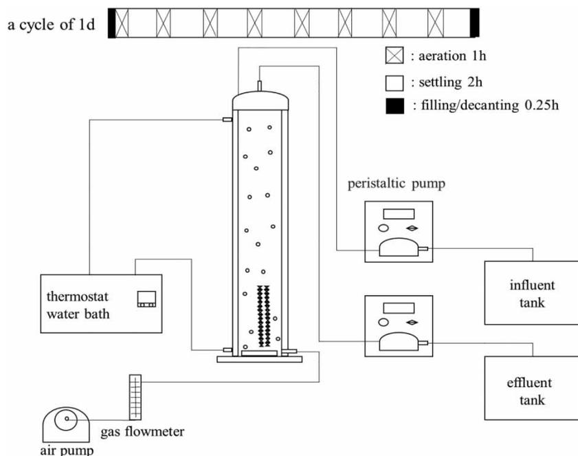
Figure 1 | Experimental set up of SBR based on ZVI.
