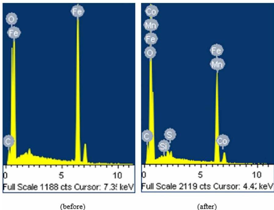
Figure 6 | Elemental composition of iron scraps before and after reaction.
