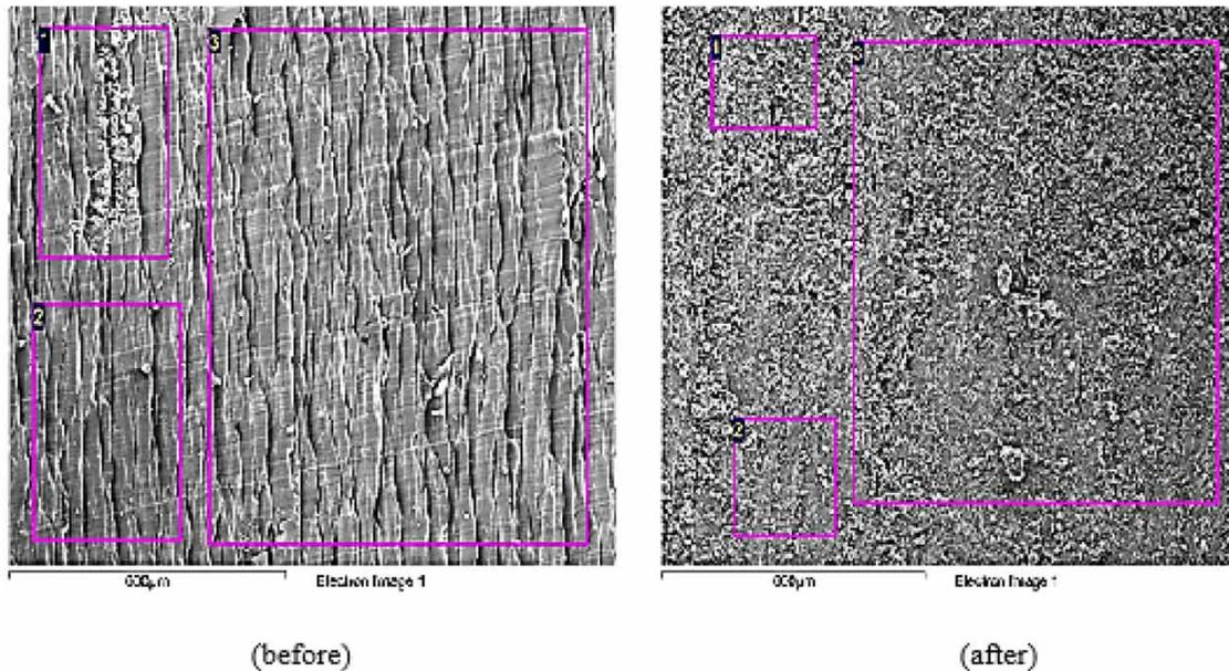
Figure 5 | Scanning electron microscope imagery of iron scraps before and after reaction.
