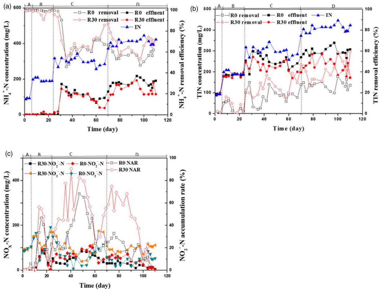
**Figure 2** | The nitrogen removal performance of SBRs without added ZVI (R0) and with added ZVI (R30): (a) concentration and removal efficiency of  $\text{NH}_4^+\text{-N}$ ; (b) concentration and removal efficiency of TIN; (c) concentration of  $\text{NO}_2^-\text{-N}$  and  $\text{NO}_3^-\text{-N}$  ( $\text{NO}_x\text{-N}$ ) and  $\text{NO}_2^-\text{-N}$  accumulation rate (NAR).
