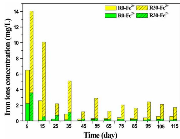
Figure 4 | Variations of  $Fe^{2+}$  and  $Fe^{3+}$  concentrations in SBRs without added ZVI (R0) and with added ZVI (R30).
