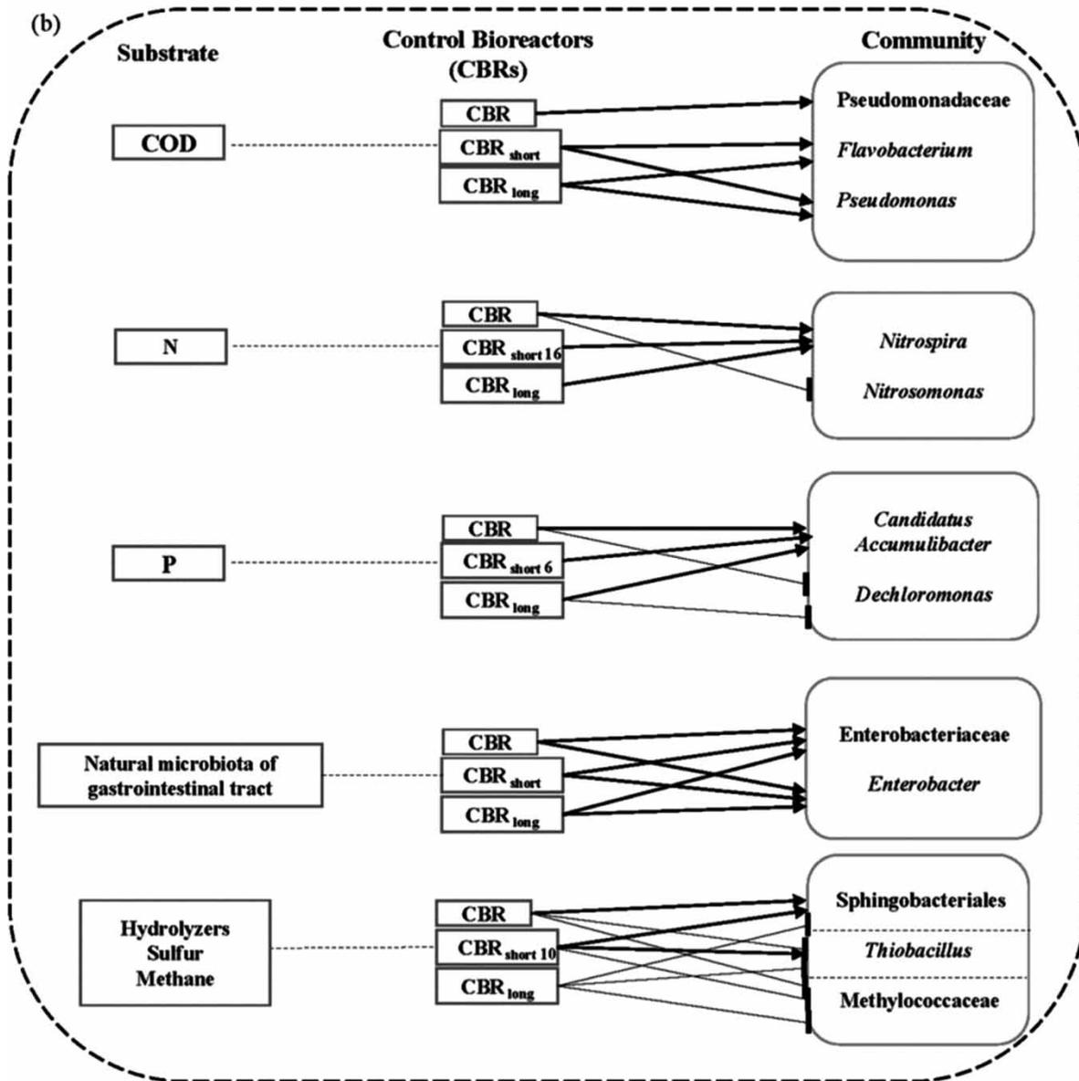
**Figure 4** | (b) Conceptual model of how different microbial species associated with the degradation of pollutants in wastewater are affected by varying HRT in CBRs. The model can be read the same way as the model for EBRs illustrated in (a).
