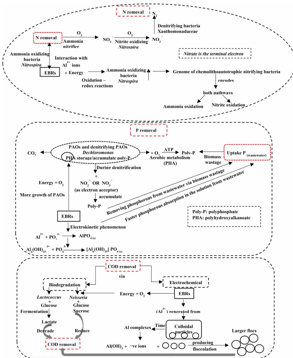
Figure 5 | Hypothetical illustration of the mechanisms of nutrient efficient removals when integrating the electrochemical process with biological treatment.
