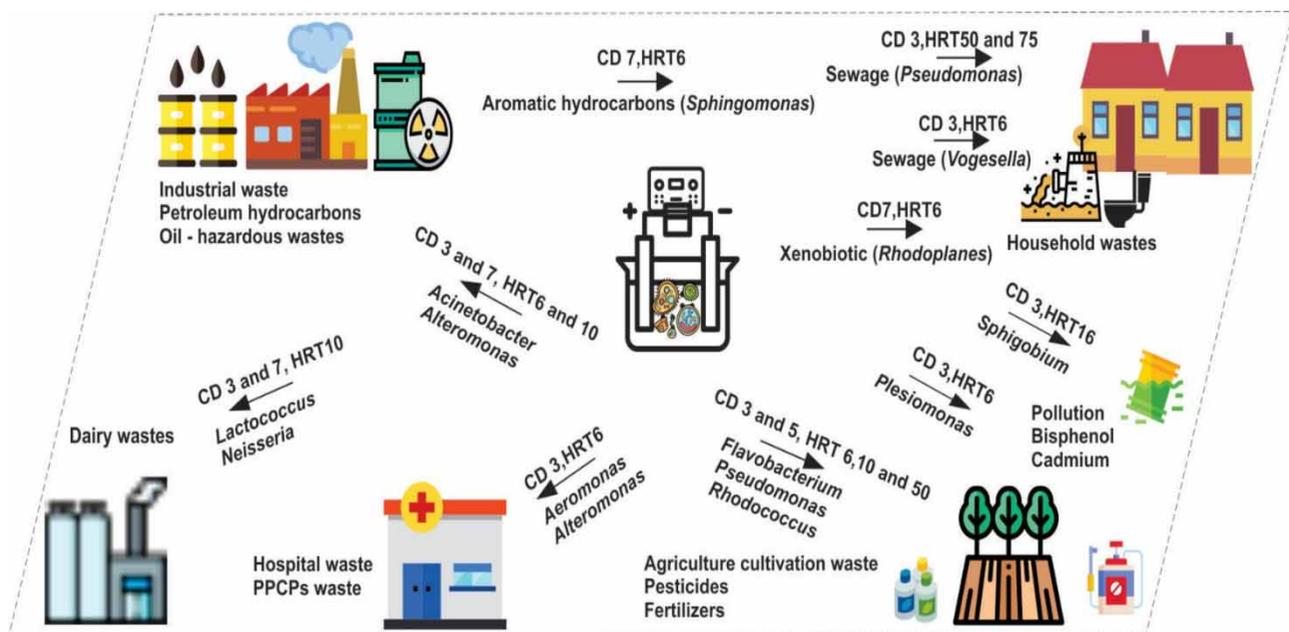
**Figure 6** | Schematic diagram showing manipulation of the operating conditions that favor functional bacteria relevant to specific types of wastewater.
