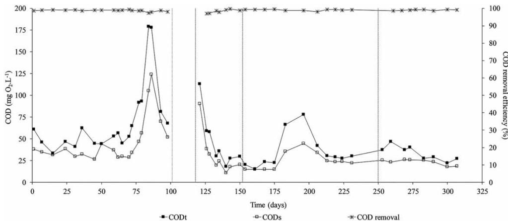
**Figure 2** | Effluent COD concentrations and COD removal efficiencies for the treatment of chocolate processing wastewater. (Dotted lines: change of operational period; day 101–119: period of mixing without feeding).
