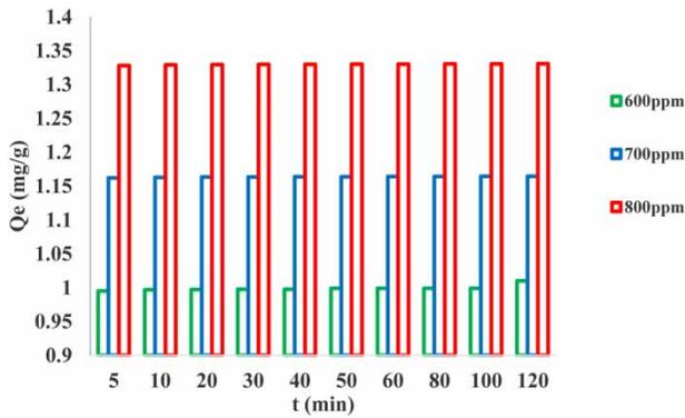
**Figure 6** | Sorption capacity of ZMLC for dye removal at variable shaking time.
