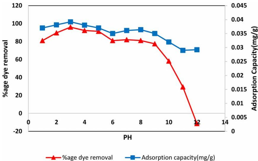
Figure 5 | Relationship between pH and ZMLC surface for gentian violet removal from aqueous media.
