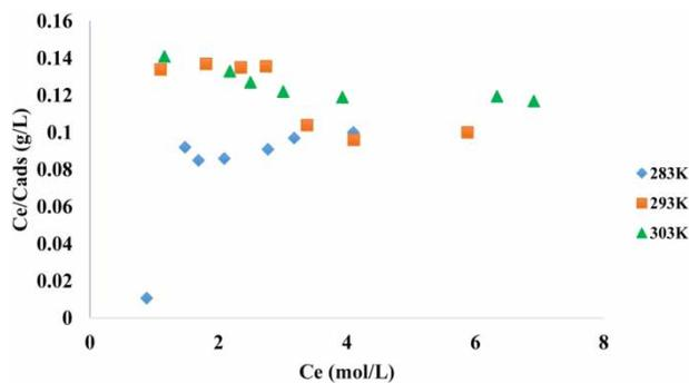
Figure 7 | Langmuir non-linear plot of ZMLC for gentian violet removal.
