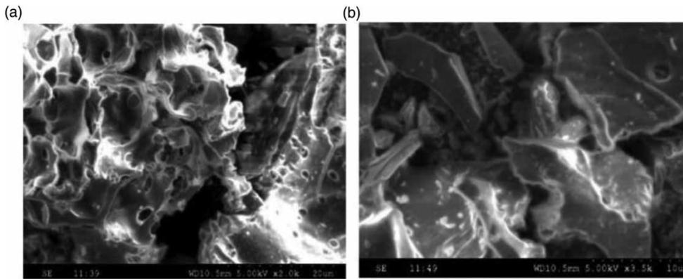
Figure 4 | SEM images of ZMLC before (a) and after (b) gentian violet adsorption.
