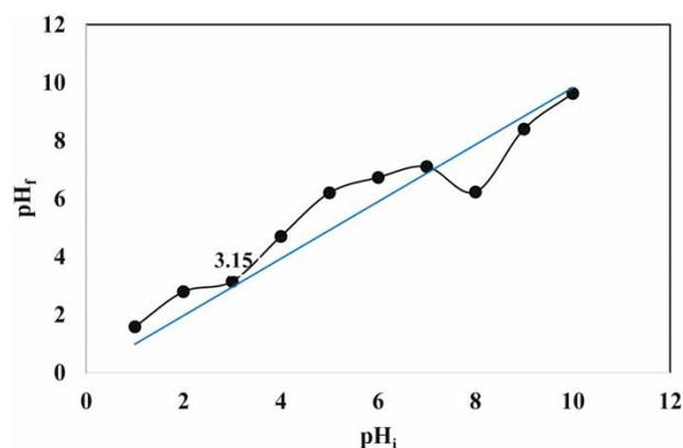
**Figure 2** | Plot for  $\text{pH}_{\text{pzc}}$  determination of ZMLC.
