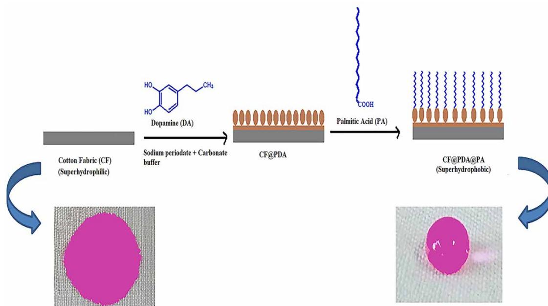
Figure 1 | Schematic diagram of the fabrication process of superhydrophobic/oleophilic cotton fabric, CF @ PDA @ PA.
