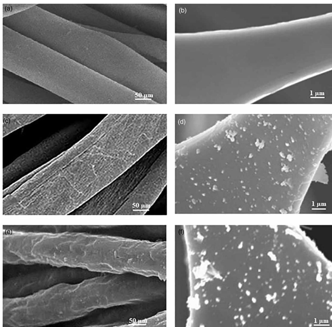
**Figure 2** | SEM images of pristine cotton fabric (a, b), modified cotton fabric with PDA (c, d), and modified cotton fabric with PDA and PA (e, f).
