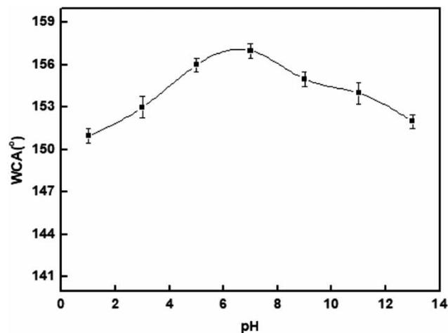
**Figure 9** | Influence of pH values of water droplet on the contact angles of the superhydrophobic cotton fabric. Error bars represent standard deviation.
