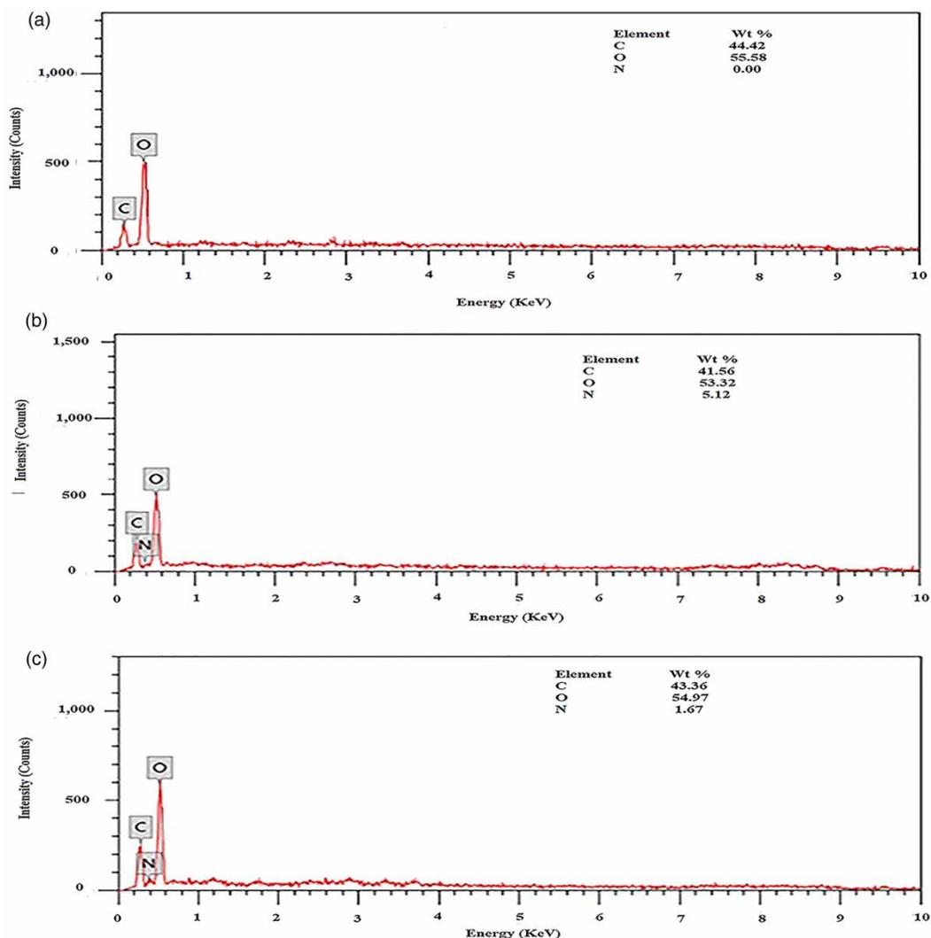
**Figure 3** | EDX analysis of the surface of pristine cotton fabric (a), modified cotton fabric with PDA (b), and modified cotton fabric with PDA and PA (c).
