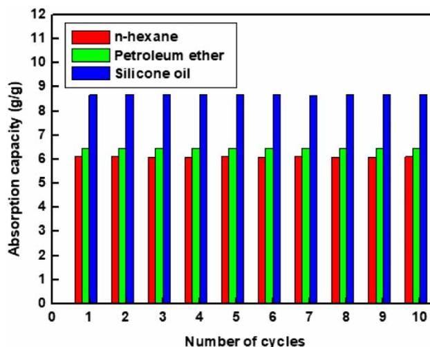
**Figure 5** | Absorption capacity for different oil/water mixtures with the number of cycles.
