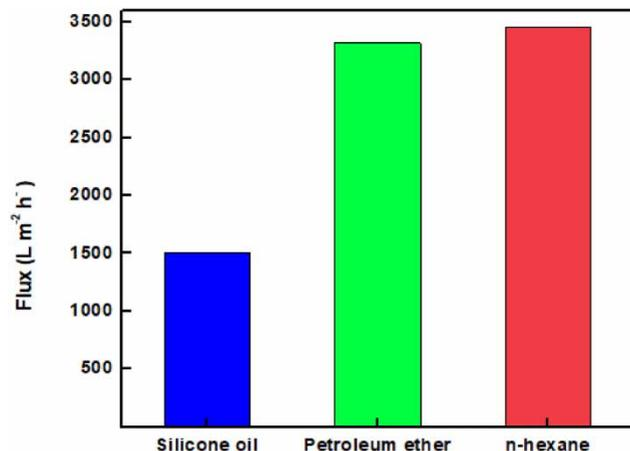
**Figure 8** | Flux values for different oil/water mixtures.
