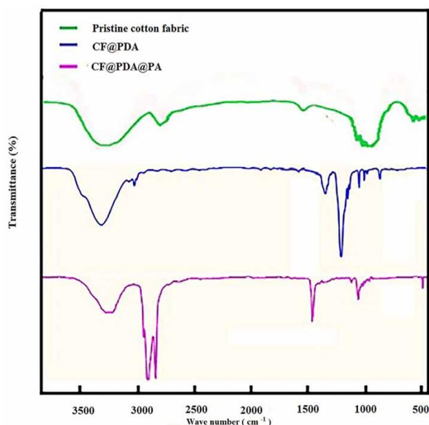
**Figure 4** | FT-IR spectra of pristine cotton, modified cotton fabric with PDA, and modified cotton fabric with PDA and PA.
