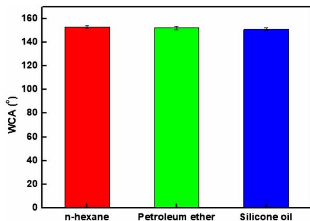
**Figure 10** | Water contact angle after 20 days' immersion of superhydrophobic cotton fabric in different oil/water mixtures. Error bars represent standard deviation.
