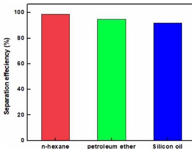
**Figure 6** | Results of separation efficiency for different oil/water mixtures.
