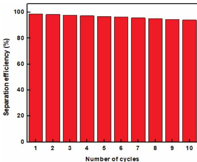
**Figure 7** | Separation efficiency for n-hexane/water mixtures with number of separation cycles.
