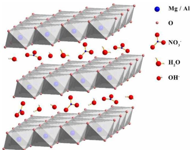
Figure 1 | The layered structure of LDHs.
