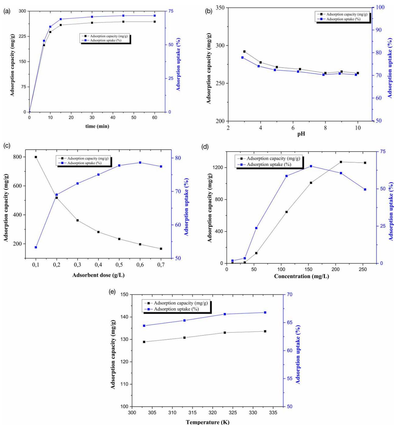
**Figure 2** | Effect of operating parameters on the adsorption uptake and capacity of MO onto MOF-5: (a) contact time, (b) initial pH, (c) adsorbent dose, (d) initial concentration of MO and (e) temperature.
