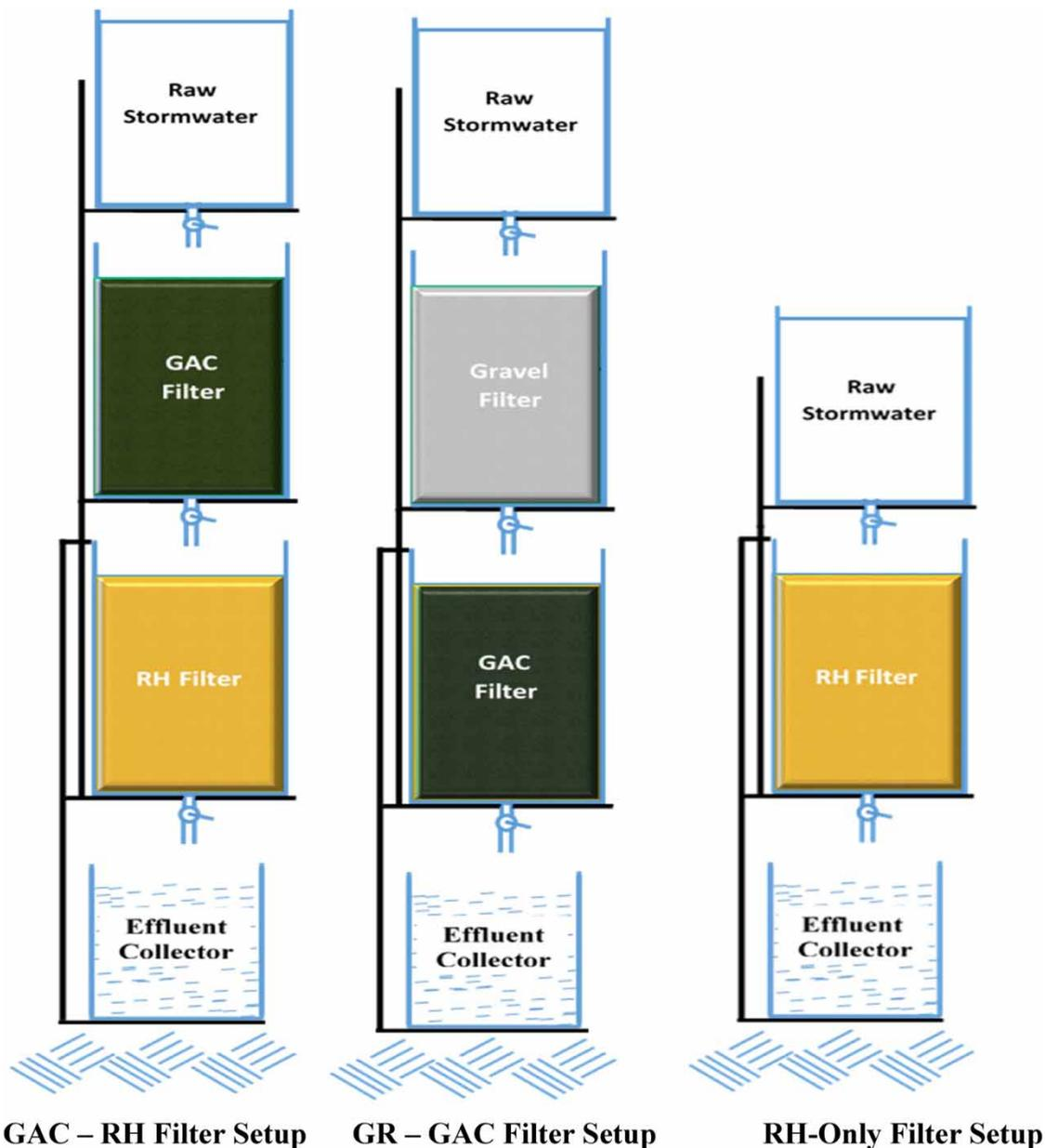
**Figure 1** | Filtration systems. GAC – RH filter, Setup GR – GAC filter setup, RH-Only filter setup.
