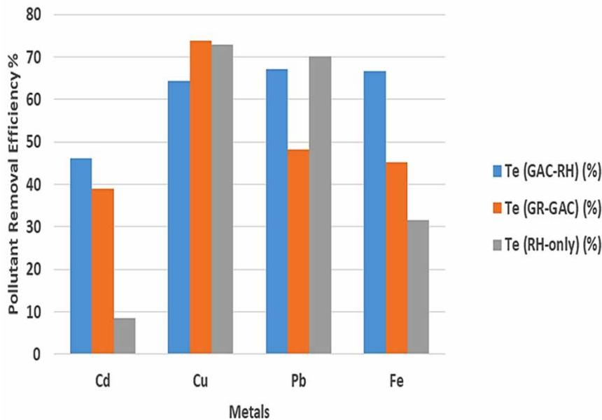
**Figure 6** | Pollutant removal efficiency of the filters.**Table 5** | Individual average workshop metal percentage removal efficiencies
