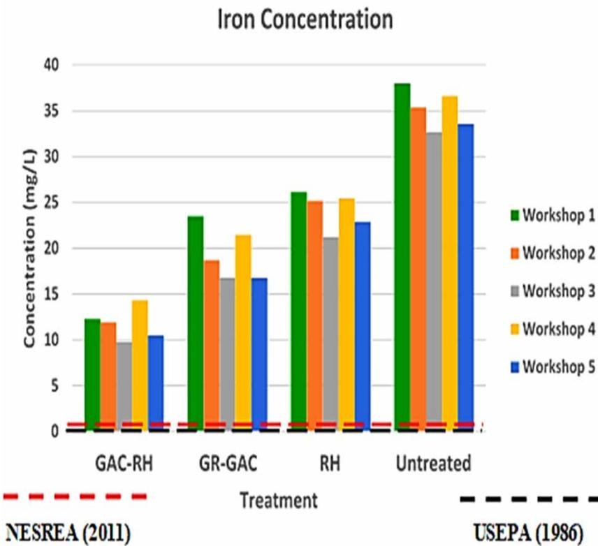
Figure 5 | Filtered and untreated Iron concentrations.
