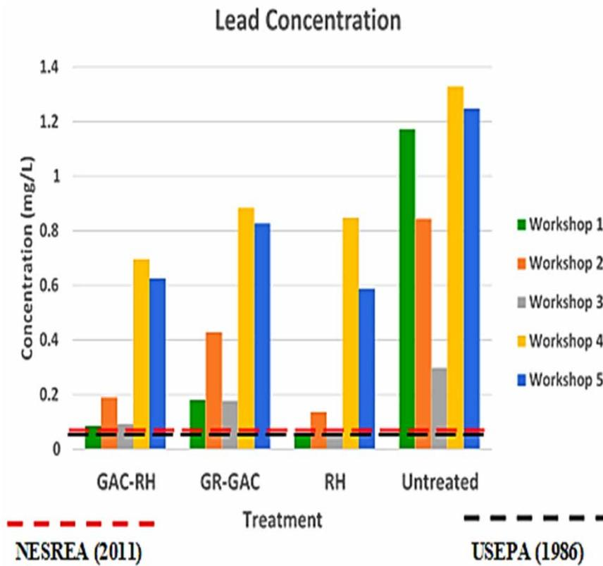
Figure 4 | Filtered and untreated lead concentrations.
