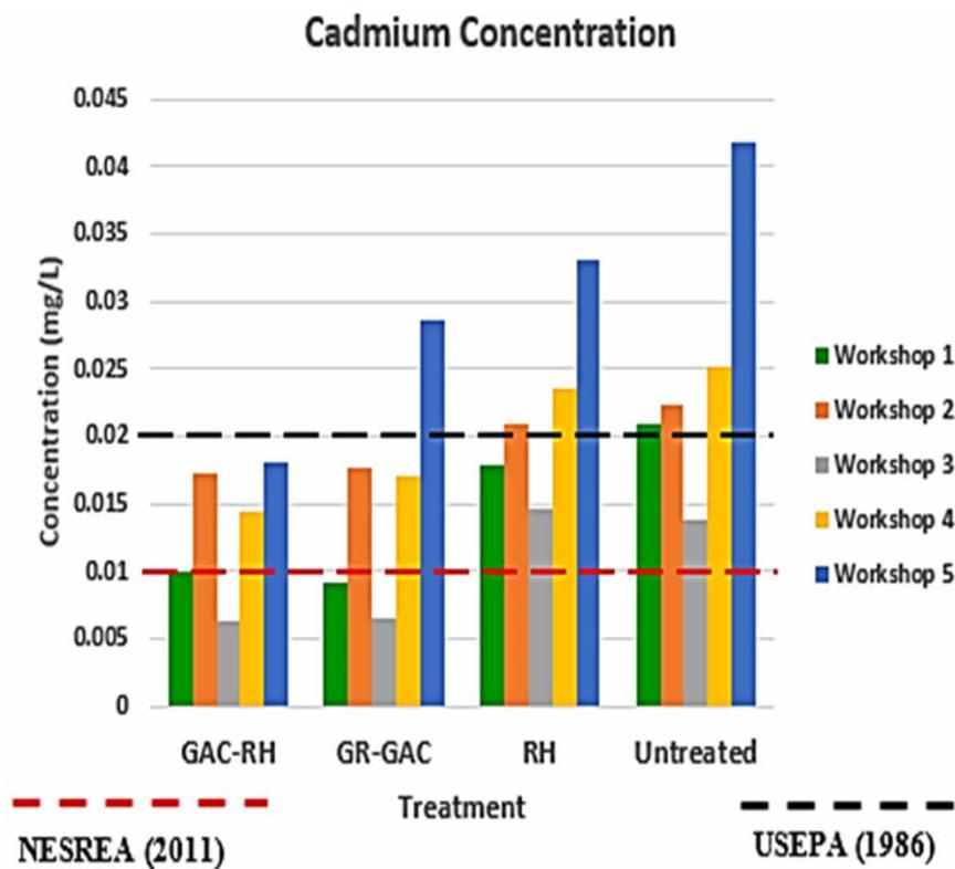
Figure 2 | Filtered and untreated cadmium concentrations.
