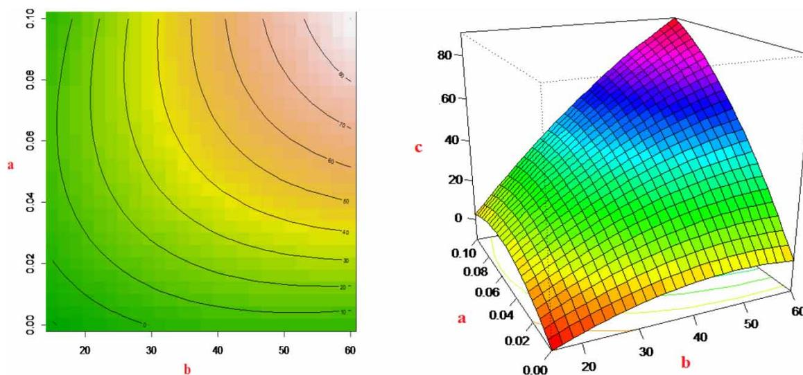
**Figure 2** | Design-expert plot: response-surface contour (left) and 3D (right) plots near the stationary point for CPF removal (%) at  $\text{pH} = 6.8 \pm 0.3$ . a: Fe-citrate/ $\text{H}_2\text{O}_2$  ratio, b: time (min) and c: removal efficiency (%).
