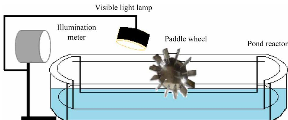
**Figure 1** | Schematic representation of the fiberglass raceway pond reactor.
