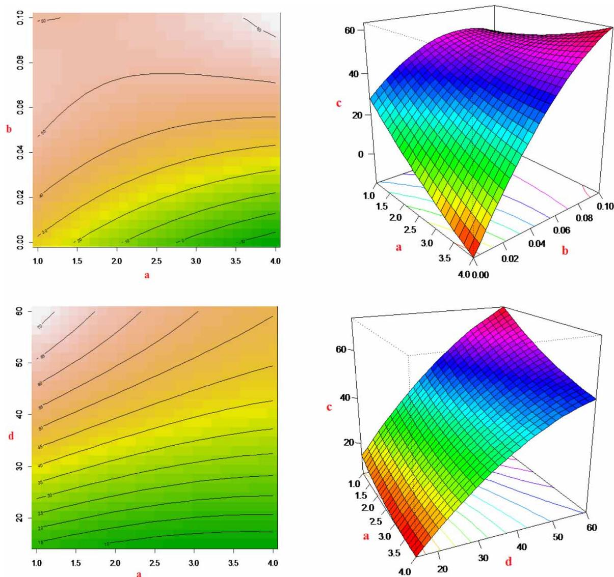
**Figure 3** | Design-expert plot: response-surface contour (left) and 3D (right) plots near the stationary point for CPF removal (%) at  $\text{pH} = 6.8 \pm 0.3$ . a: Initial CPF concentration ( $\text{mg L}^{-1}$ ), b: Fe-citrate/ $\text{H}_2\text{O}_2$  ratio, c: removal efficiency (%) and d: time (min).
