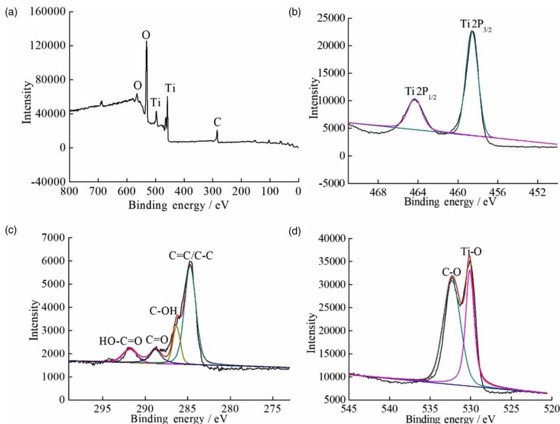
**Figure 2** | XPS spectra of graphene-doped TiO<sub>2</sub> microspheres.
