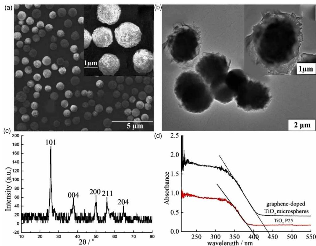
**Figure 1** | Characterization results of the graphene-doped TiO<sub>2</sub> microspheres: (a) SEM, (b) TEM, (c) XRD, (d) UV-Vis DRS.
