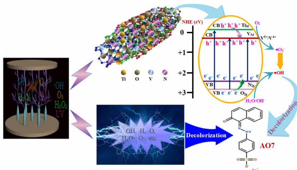
**Figure 12** | The proposed mechanism of synergistic effect of pulsed discharge plasma and V/N-TiO<sub>2</sub>-MWCNTs composite for AO7 removal from aqueous solution.
