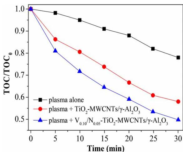
**Figure 11** | The changes of TOC after different discharge plasma treatment times with V<sub>0.10</sub>/N<sub>0.05</sub>-TiO<sub>2</sub>-MWCNTs composite.
