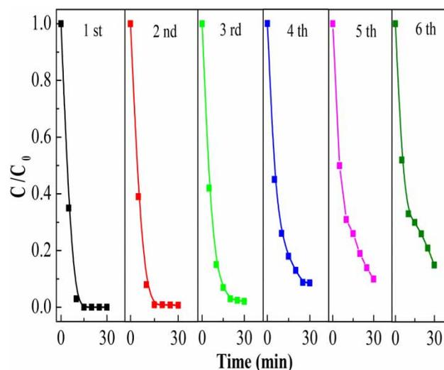
**Figure 7** | Recyclability studies of the V/N-TiO<sub>2</sub>-MWCNTs composite for AO7 removal in pulsed discharge plasma system.
