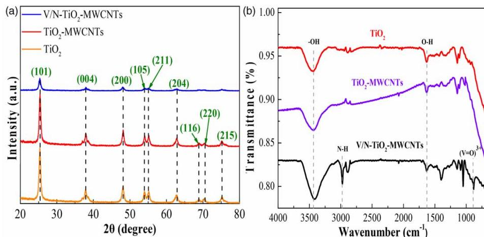
Figure 1 | XRD (a) and FTIR (b) spectra of prepared TiO<sub>2</sub>, TiO<sub>2</sub>-MWCNTs and V/N-TiO<sub>2</sub>-MWCNTs composites.
