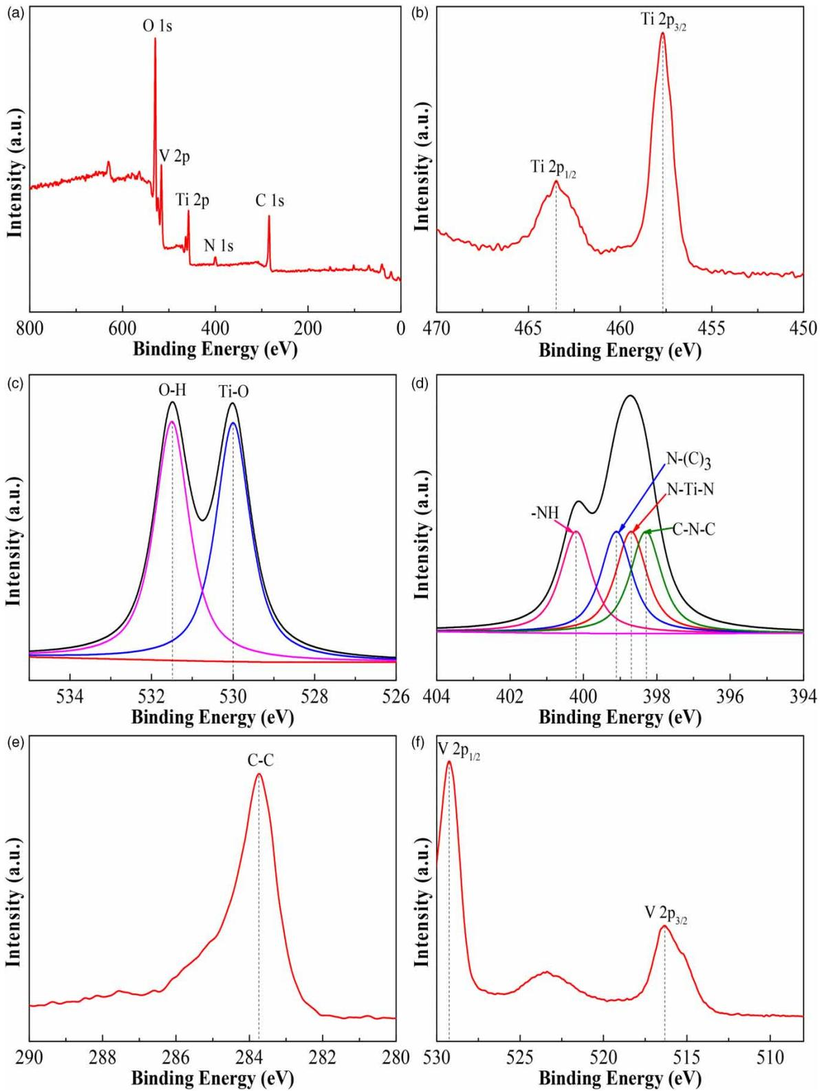
**Figure 3** | XPS fully scanned spectra of V/N-TiO<sub>2</sub>-MWCNTs composite (a), XPS spectra of Ti 2p (b), XPS spectra of O 1s (c), XPS spectra of N 1s (d), XPS spectra of C 1s (e) and XPS spectra of V 2p (f).
