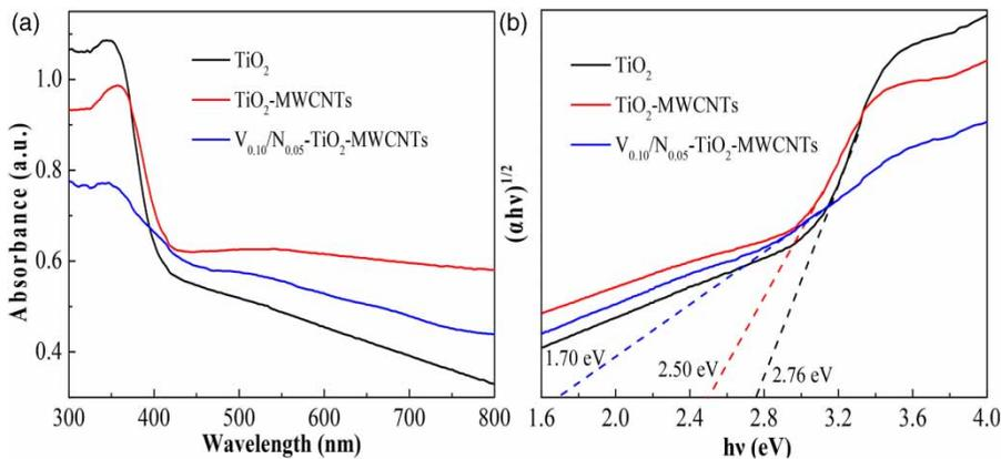
**Figure 8** | UV-Vis spectra (a) and plots of  $(\alpha hv)^{1/2}$  vs photon energy (b) of the prepared  $\text{TiO}_2$ ,  $\text{TiO}_2$ -MWCNTs and  $\text{V}_{0.10}/\text{N}_{0.05}$ - $\text{TiO}_2$ -MWCNTs composites.
