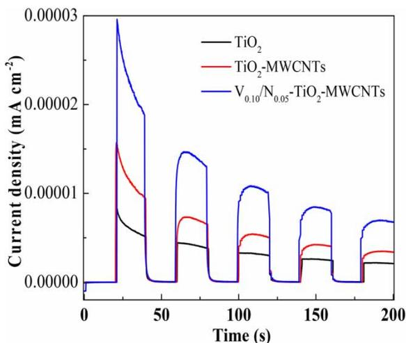
**Figure 9** | The photocurrent response curves of the photoelectrodes consisting of  $\text{TiO}_2$ ,  $\text{TiO}_2$ -MWCNTs and  $\text{V}_{0.10}/\text{N}_{0.05}$ - $\text{TiO}_2$ -MWCNTs composites.
