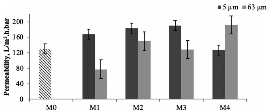
**Figure 3** | Pure water permeability of 5 and 63  $\mu\text{m}$  of HNT membranes.
