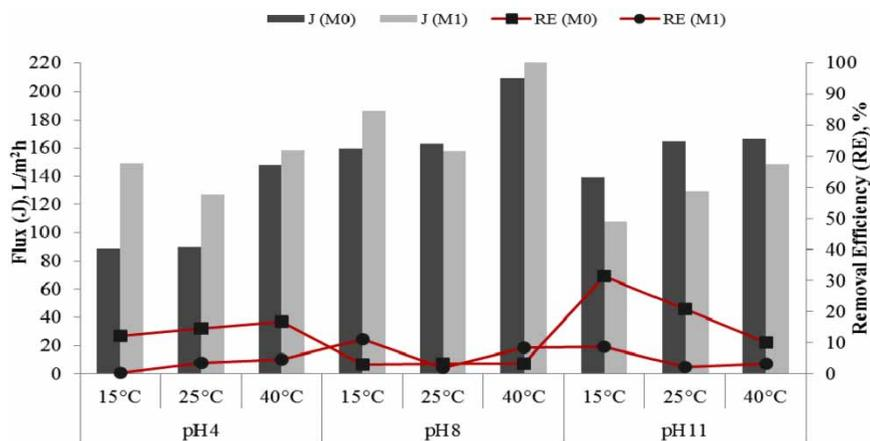
Figure 7 | Reactive Orange dye flux and removal efficiency of M0 and M1 membranes at three different temperatures and pH values.
