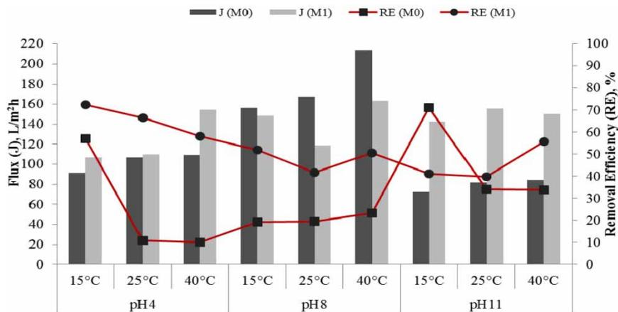
Figure 6 | Setazol Red dye flux and removal efficiency of M0 and M1 membranes at three different temperatures and pH values.
