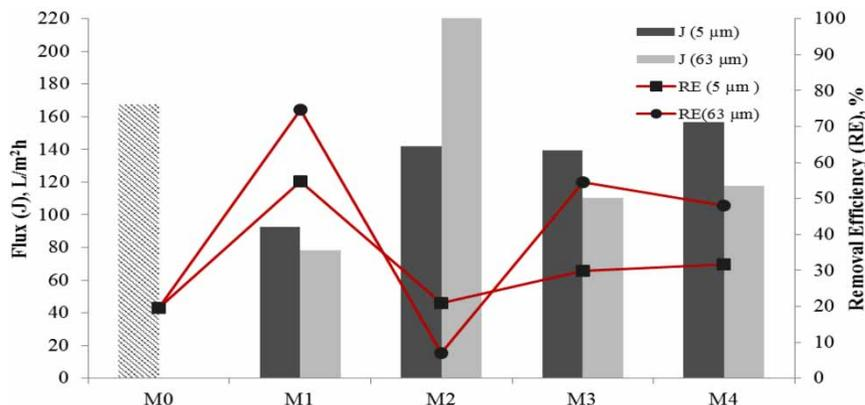
Figure 4 | Setazol Red dye flux and removal efficiency of membranes.
