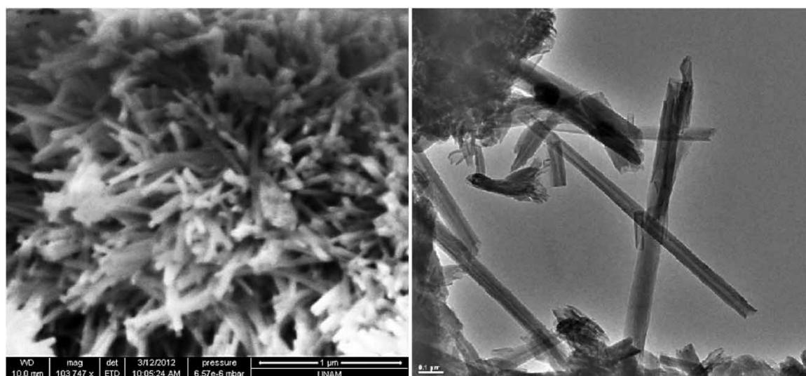
**Figure 2** | SEM and TEM images of 5  $\mu\text{m}$  after milled HNT.
