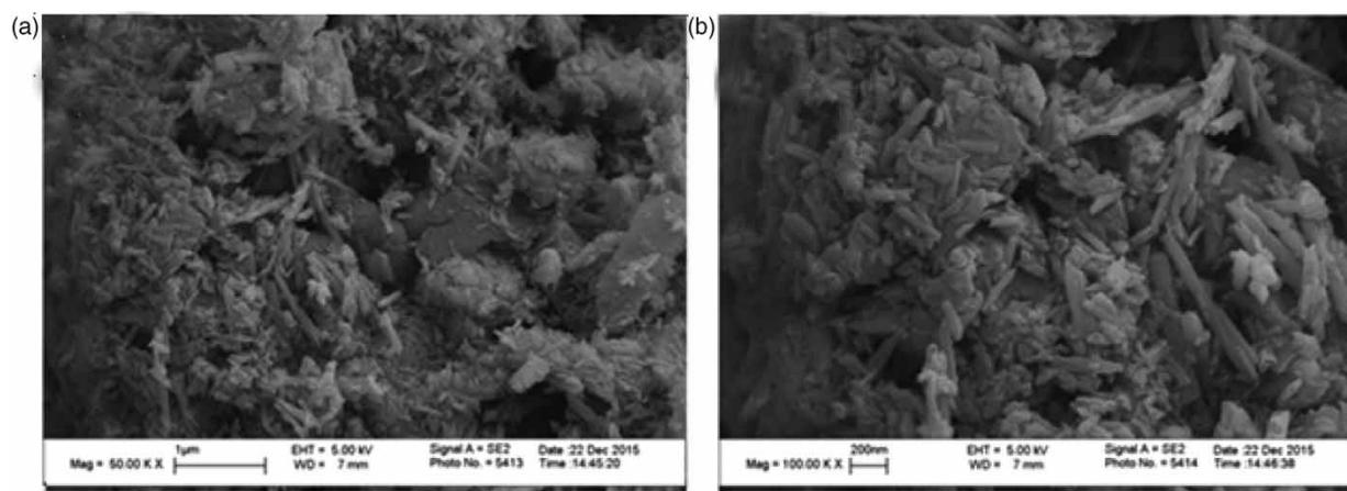
**Figure 1** | SEM images of HNT (a: 5  $\mu\text{m}$  after milled HNTs, b: 63  $\mu\text{m}$  original HNTs).
