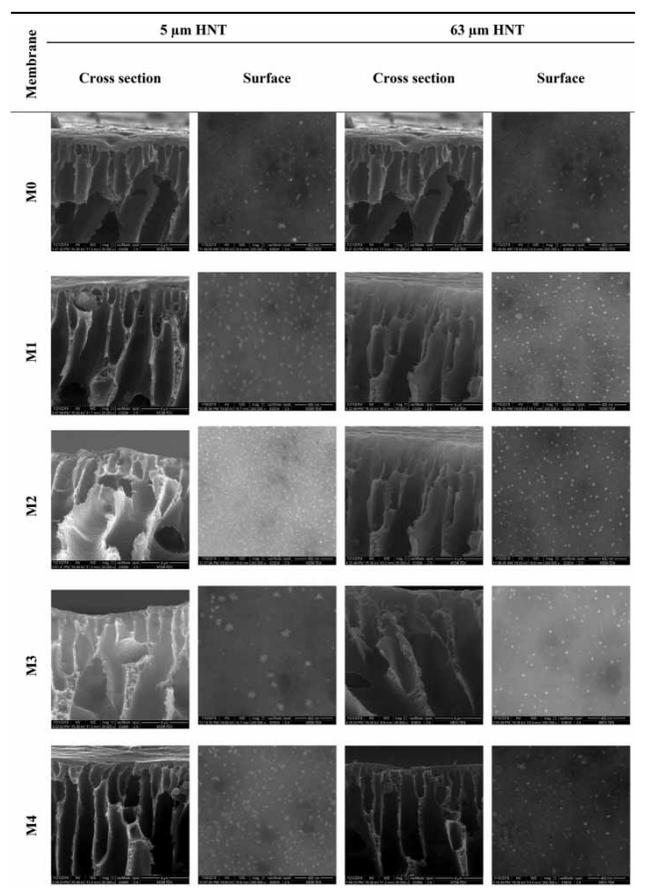
a recent study, Zeng *et al.* (2017) used modified HNTs with dopamine and they fabricated PVDF nanocomposite membranes by using different ratios of functionalized HNT. According to SEM images, there were no particular changes between the surface morphology of pristine PVDF membrane and HNT incorporated membranes. On the other hand, the addition of D-A-modified HNT resulted in the gradual increase of microcavities in membrane structure and
