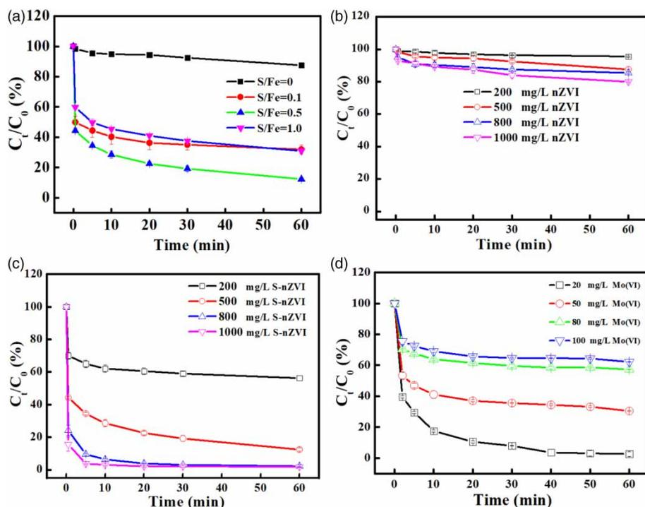
**Figure 1** | Effect of (a) nZVI with different S/Fe molar ratios (50 mg/L Mo(VI), 500 mg/L S-nZVI), (b) initial nZVI dose (50 mg/L Mo(VI)), (c) initial S-nZVI dose (50 mg/L Mo(VI), S/Fe molar ratio = 0.5), and (d) initial Mo(VI) concentration (500 mg/L S-nZVI, S/Fe ratio = 0.5) on Mo(VI) removal at pH = 7.0 and T = 25 °C; error bars present mean  $\pm$  standard deviation).
