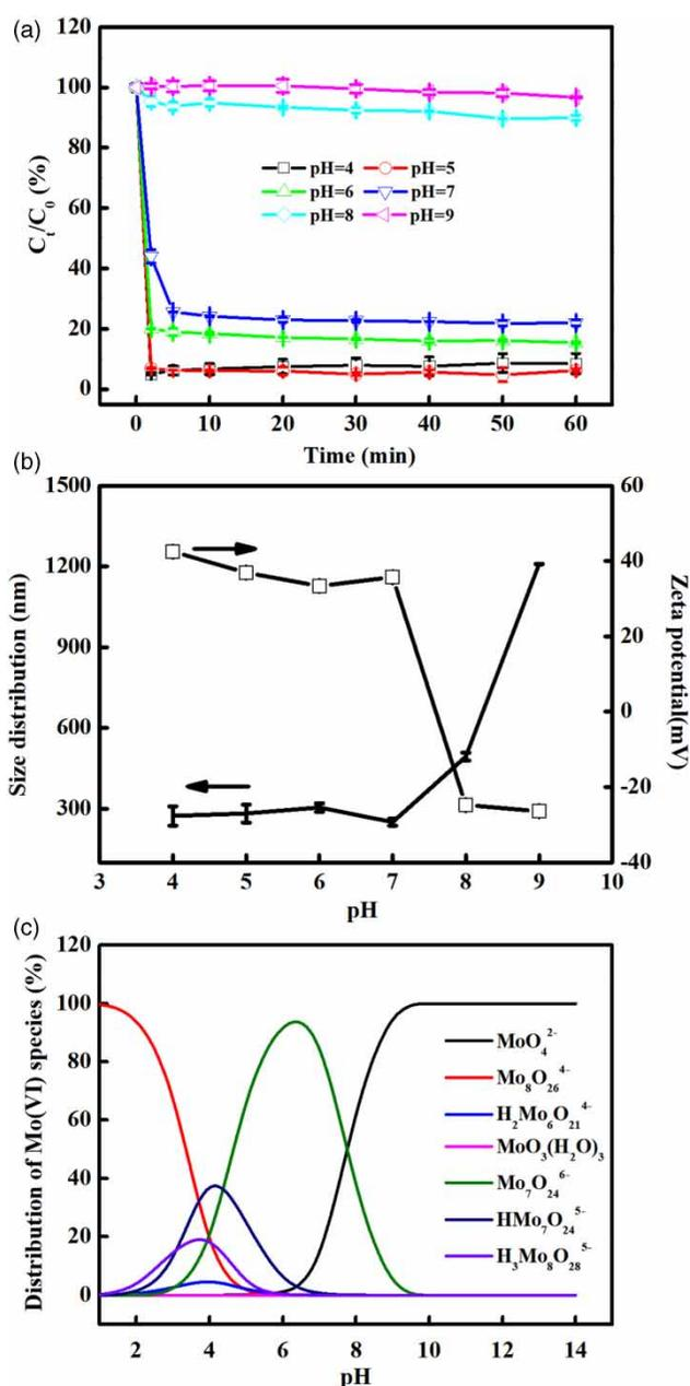
**Figure 4** | Effect of pH on (a) Mo(VI) removal by S-nZVI (50 mg/L Mo(VI), 500 mg/L S-nZVI, S/Fe molar ratio = 0.5), (b) size distribution and zeta potential of S-nZVI with 0.5 molar ratio of S/Fe, and (c) distribution of Mo(VI) species (Mo(VI) concentration = 50 mg/L, T = 25 °C, ion strength = 0.1 M  $\text{KNO}_3$ ); error bars present mean  $\pm$  standard deviation.
