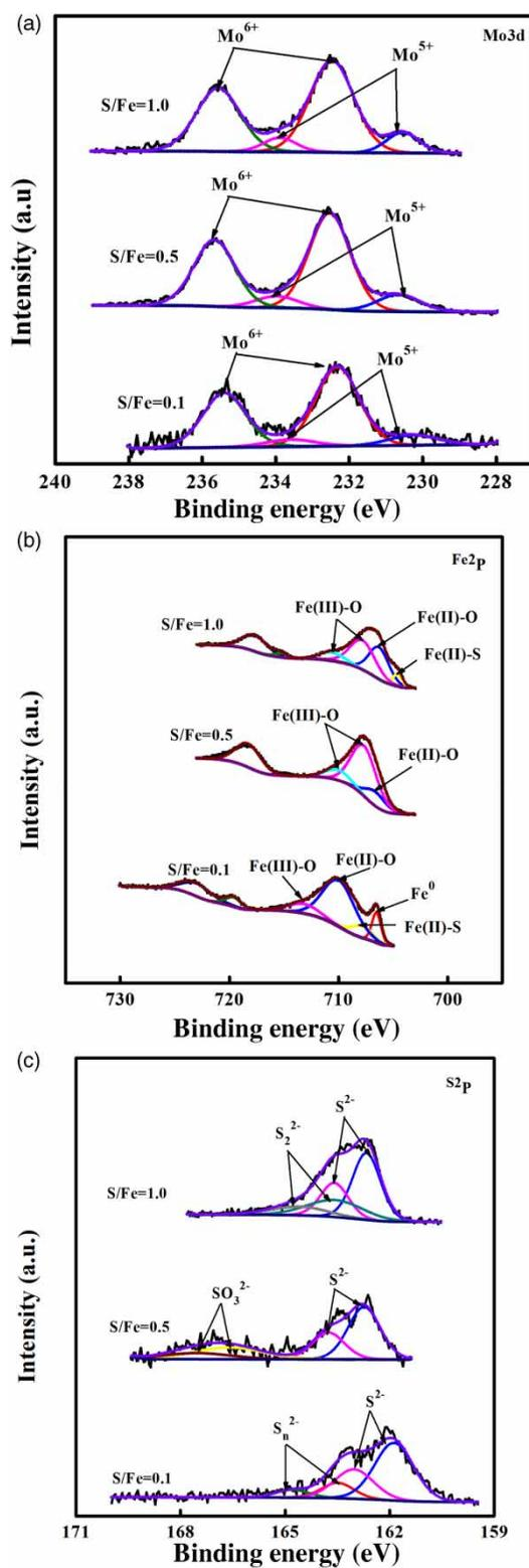
**Figure 3** | XPS spectra of Mo(VI) treated with S-nZVI with different S/Fe ratios, and narrow scans of (a) Mo3d, (b) Fe2p, (c) S2p (50 mg/L Mo(VI), 500 mg/L S-nZVI 0.5 molar ratio of S/Fe, pH = 7.0, black and purple represent the original and the sum total of other colored lines, respectively). Please refer to the online version of this paper to see this figure in color: <http://dx.doi.org/10.2166/wst.2020.570>.
