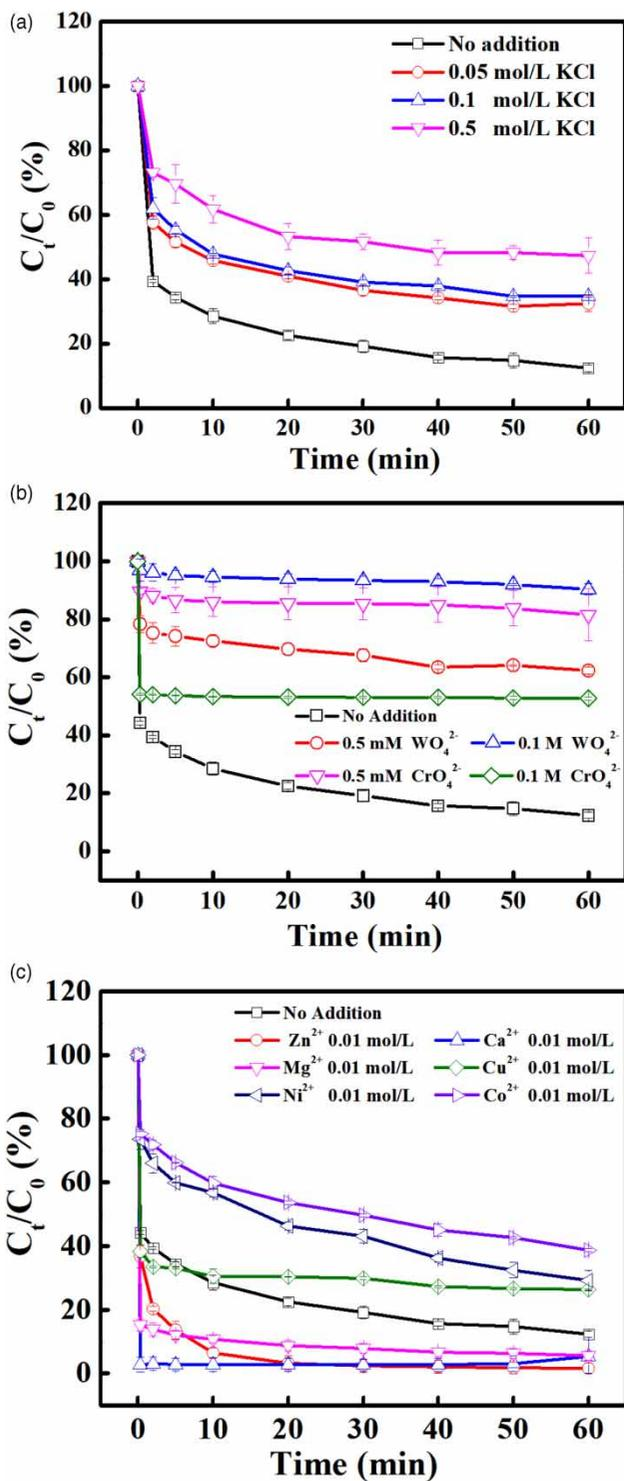
**Figure 5** | Effect of (a) KCl concentration, (b) competing anions, (c) co-existing cations on Mo(VI) removal by S-nZVI ( $T = 25\text{ }^{\circ}\text{C}$ ,  $\text{pH} = 7.0$ ,  $50\text{ mg/L Mo(VI)}$ ,  $500\text{ mg/L S-nZVI}$  with 0.5 molar ratio of S/Fe, error bars present mean  $\pm$  standard deviation).
