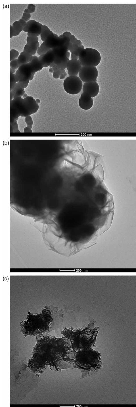
**Figure 2** | TEM images of (a) unmodified nZVI, (b) S-nZVI<sub>0.5</sub> before the reaction with Mo(VI), and (c) S-nZVI<sub>0.5</sub> after the reaction with Mo(VI) (50 mg/L Mo(VI), 500 mg/L S-nZVI, S/Fe molar ratio = 0.5, pH = 7.0).
