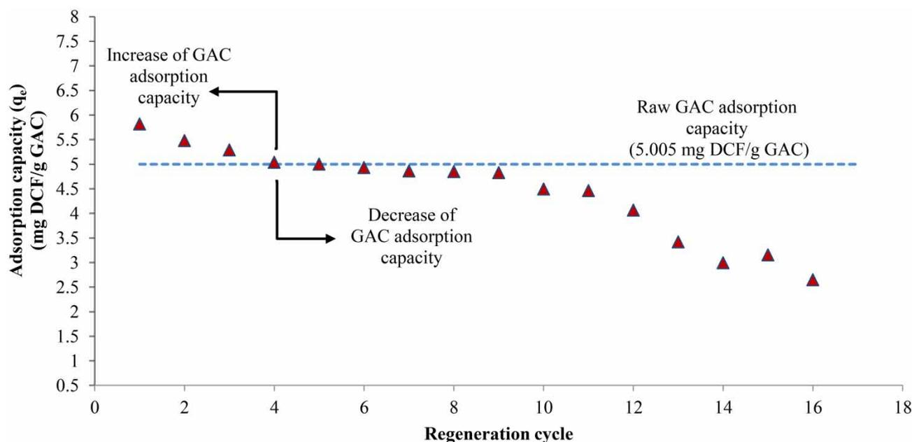
Figure 2 | Change of the adsorption capacity of regenerated GAC against the regeneration cycle.
