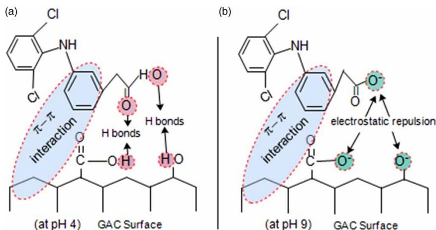
**Figure 5** | Possible mechanism of DCF adsorption on GAC.
