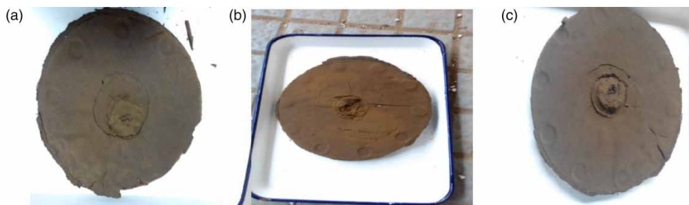
Figure 14 | Sludge filter cakes by filter press in verification test (a: batch 1, b: batch 2, c: batch 3).
