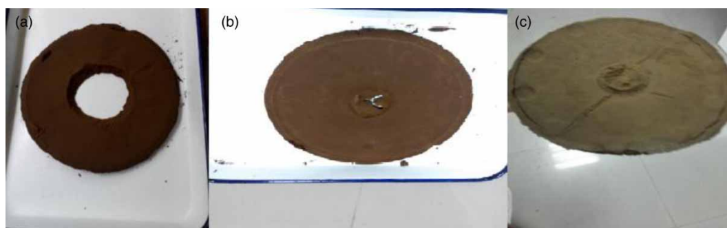
Figure 13 | The pictures of the seventh (a), fifth (b) and third (c) batches of sludge filter cake.
