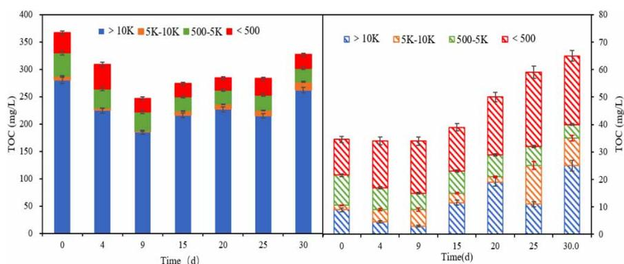
Figure 9 | Variation of total TOC and different molecular weight of TOC (solid line: 100% sludge extract; dotted line: BG11).
