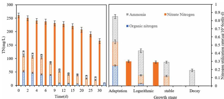
**Figure 7** | Comparison of utilization and utilization rate of N by *C. vulgaris* in BG11 (solid line: BG11; dotted line: 100% sludge extract).
