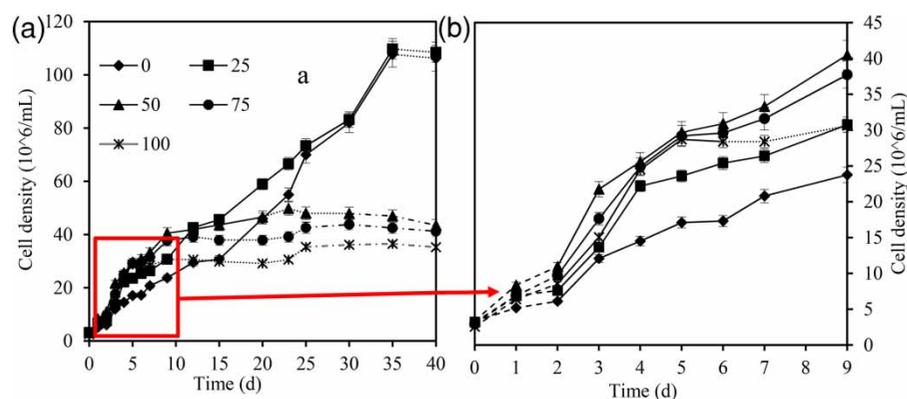
**Figure 2** | The variation of cell density of *C. vulgaris* cultured in sludge extracts diluted by BG11 with the different dilution ratios. (a) The whole-cell density; (b) cell density on days 0–9.
