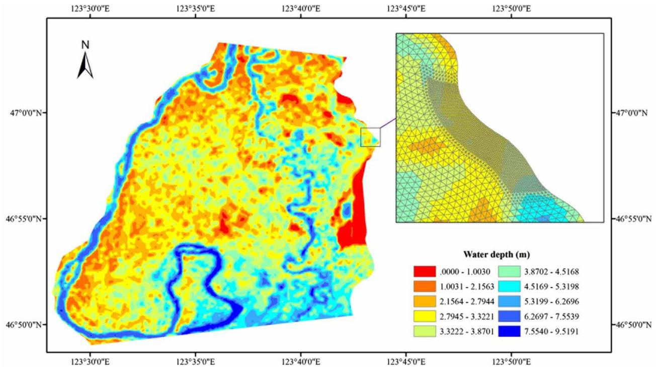
**Figure 5** | The water depth grid of the once-in-50-year flood in the research area and the partial enlarged image of the vegetation area.
