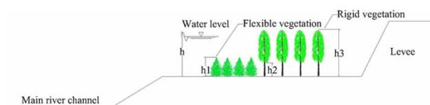
Figure 8 | Design of combined-vegetation wave break forest.
