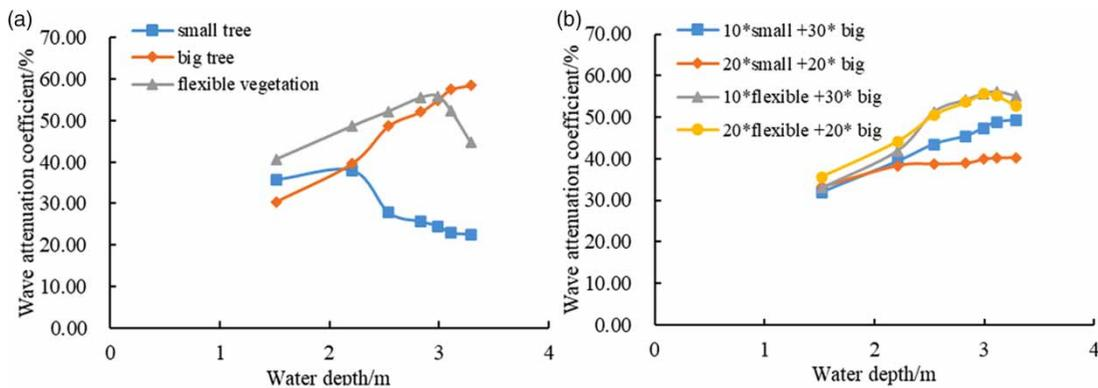
**Figure 7** | Wave attenuation coefficients of different single-vegetation forests (a) and combined-vegetation forests (b).
