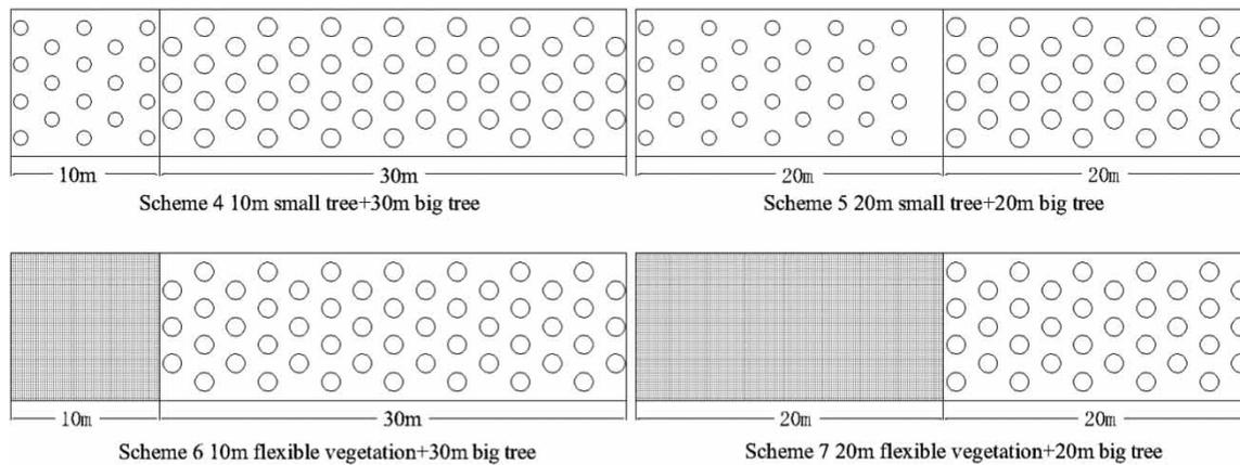
**Figure 2** | Sketch of the four combined-vegetation schemes.**Table 3** | Experimental water depth conditions
