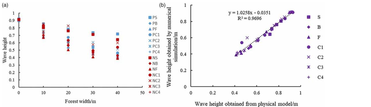
**Figure 6** | Wave height of each measuring position for the water level of a 50-year return period (a) and the comparison of results between physical experiments and numerical simulations (b). In the legend, P = physical experiment, N = numerical simulation, S = small tree scheme, B = big tree, F = flexible vegetation and C = combined-vegetation forests.
