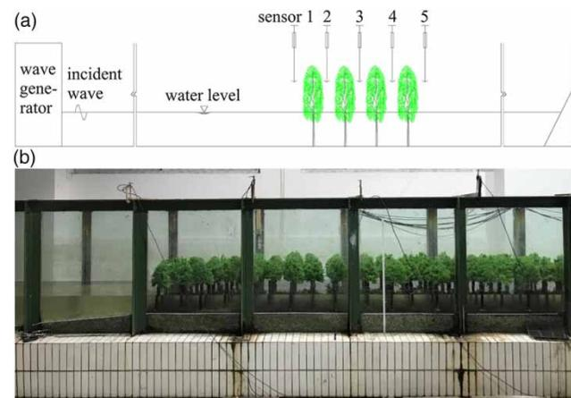
**Figure 3** | Sketch of experimental channel layout (a) and side view of experimental scenery (b).
