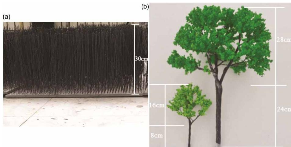
**Figure 4** | Flexible model vegetation (a) and rigid model trees (b).
