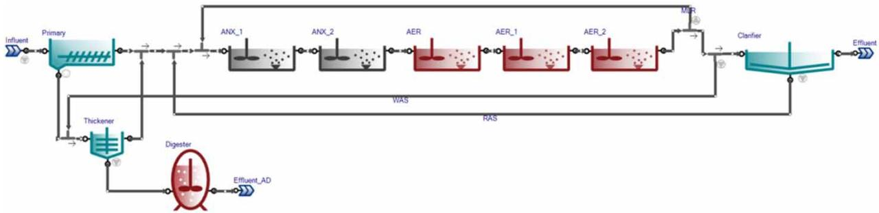
**Figure 2** | Schematic of MLE nitrogen removal process.
