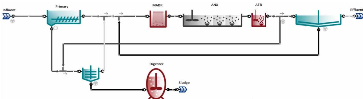
Figure 1 | Schematic of hybrid MABR biological nitrogen removal process.
