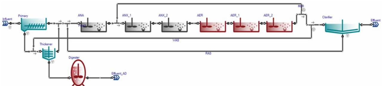
**Figure 4** | Schematic of A<sup>2</sup>/O N&P removal process.
