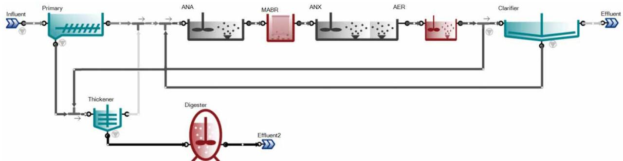
**Figure 3** | Schematic of hybrid MABR biological nitrogen and phosphorus removal process.
