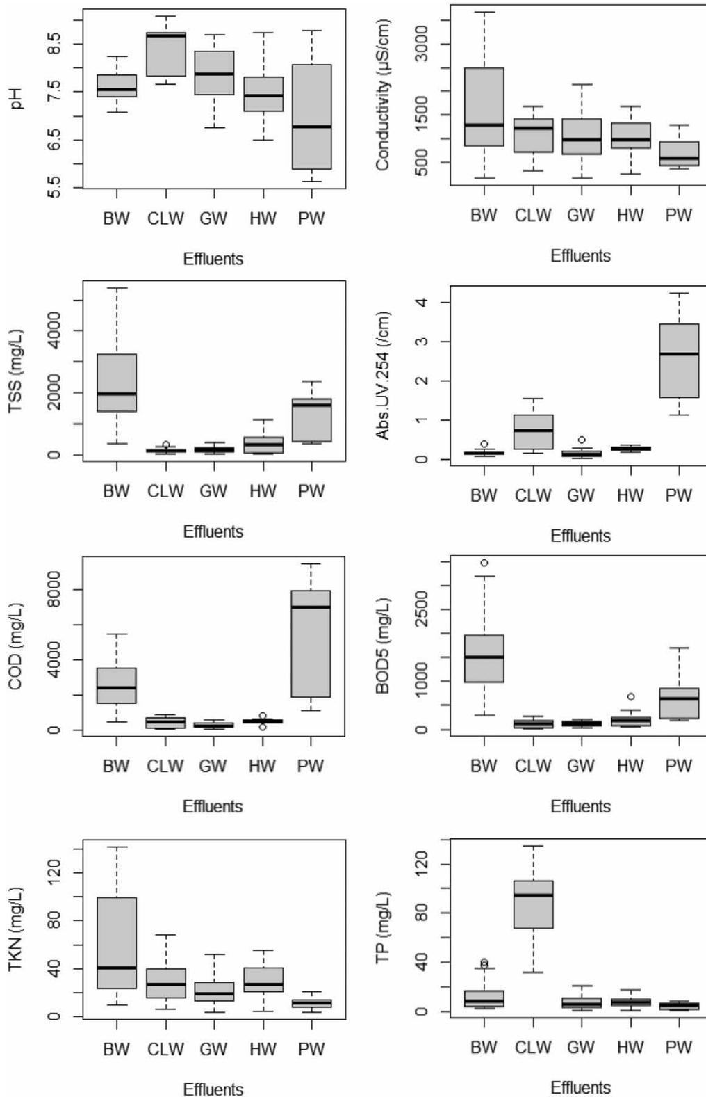
**Figure 2** | Distribution of the values of physicochemical parameters of different effluents. BW: Blackwater, CLW: Commercial laundry wastewater, GW: Greywater, HW: Hospital wastewater, PW: Pharmaceutical wastewater.
