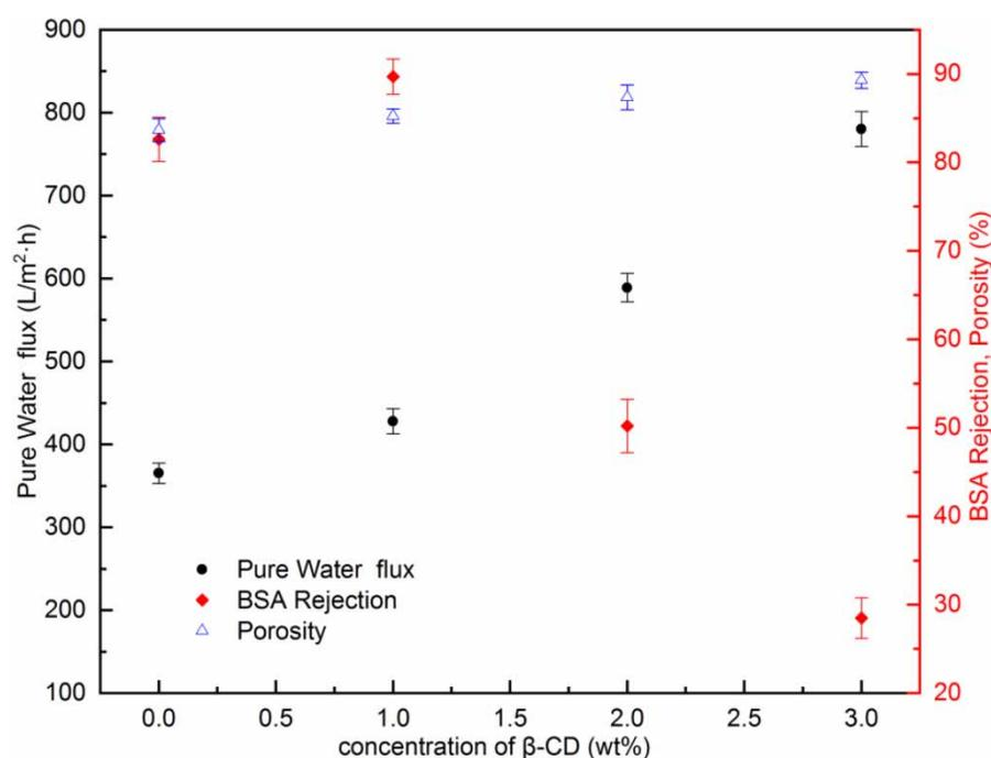
Figure 5 | Variations in water flux, retention rate and porosity of PVDF/PMMA five-bore HFMs with different  $\beta$ -CD concentrations (PVDF:PMMA = 80:20, 5 wt.% PVP).
