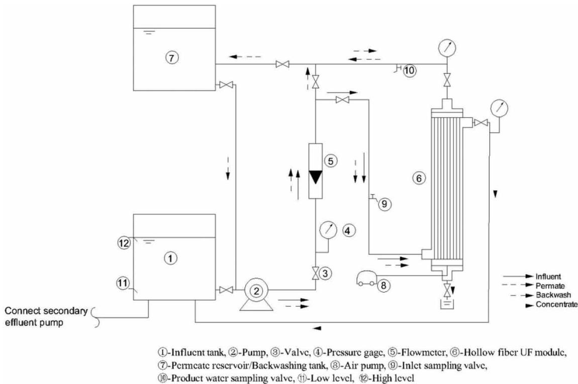
**Figure 4** | Schematic of advanced treatment of dyeing wastewater.
