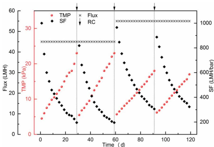
**Figure 10** | Variation in TMP, flux, and SF in influent and effluent.
