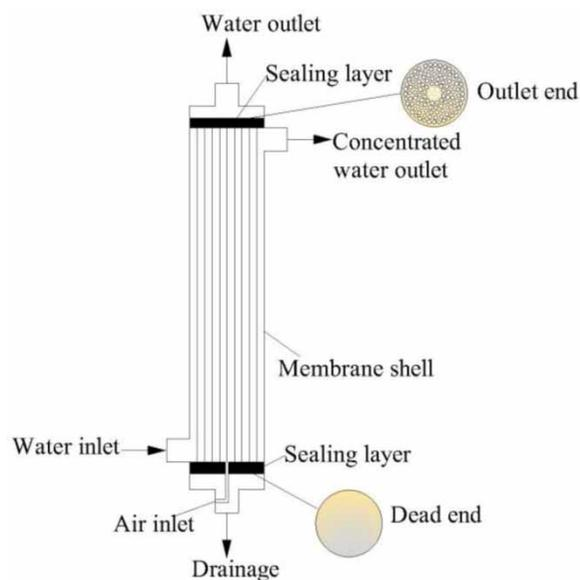
Figure 3 | The laboratory made membrane module.
