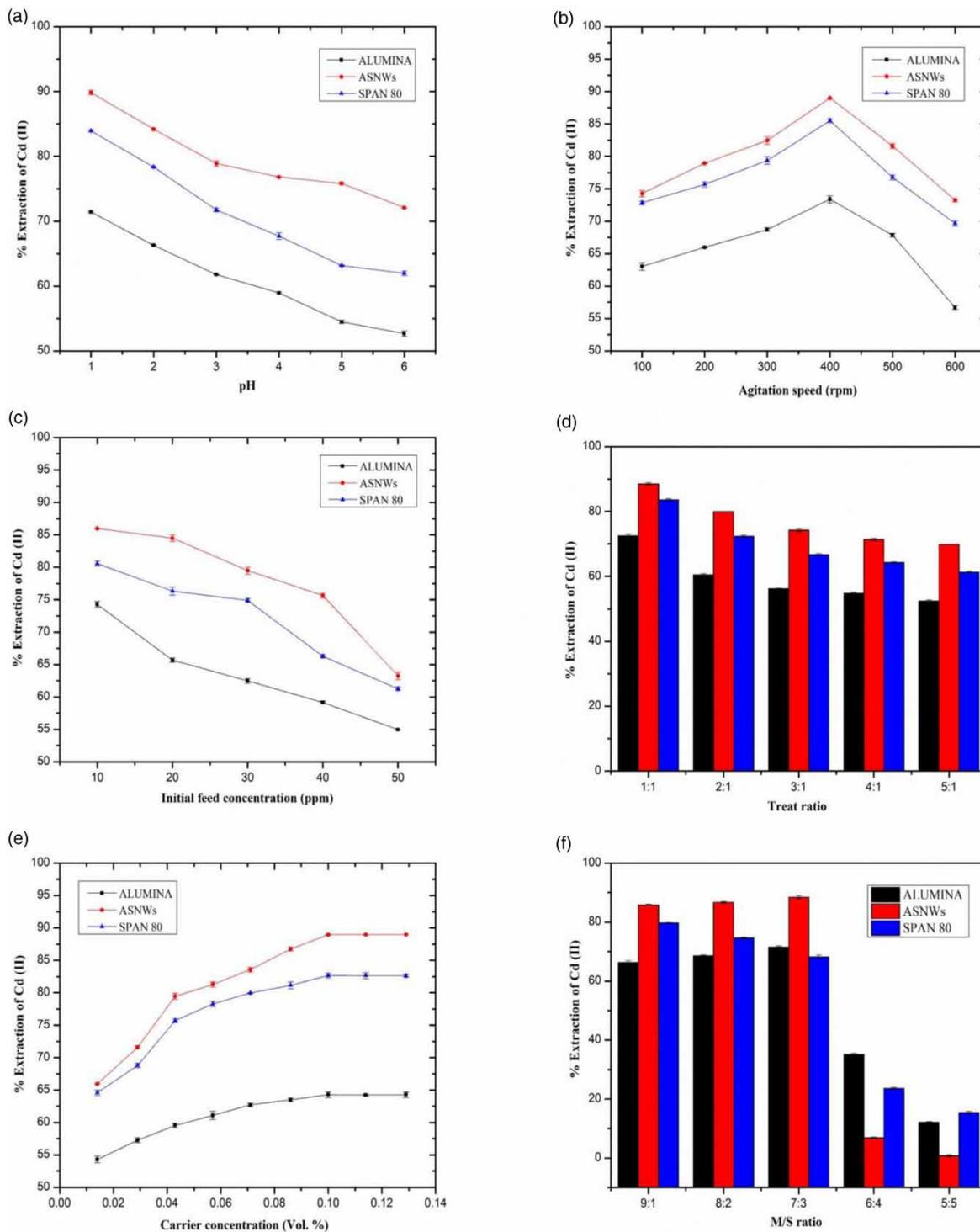
**Figure 4** | Effect of various parameters on percentage extraction of Cd (II) (a) pH, (b) agitation speed, (c) initial feed concentration, (d) treat ratio, (e) carrier concentration and (f) M/S ratio.
