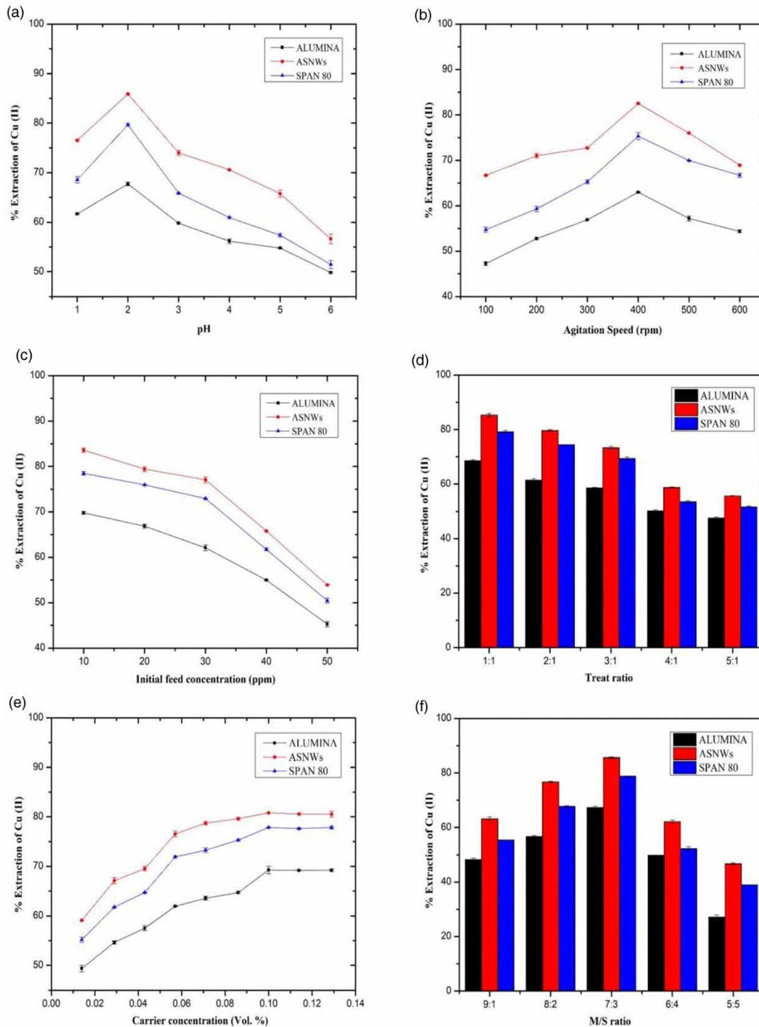
**Figure 1** | Effect of various parameters on percentage extraction of Cu (II) (a) pH, (b) agitation speed, (c) initial feed concentration, (d) treat ratio, (e) carrier concentration and (f) M/S ratio.
