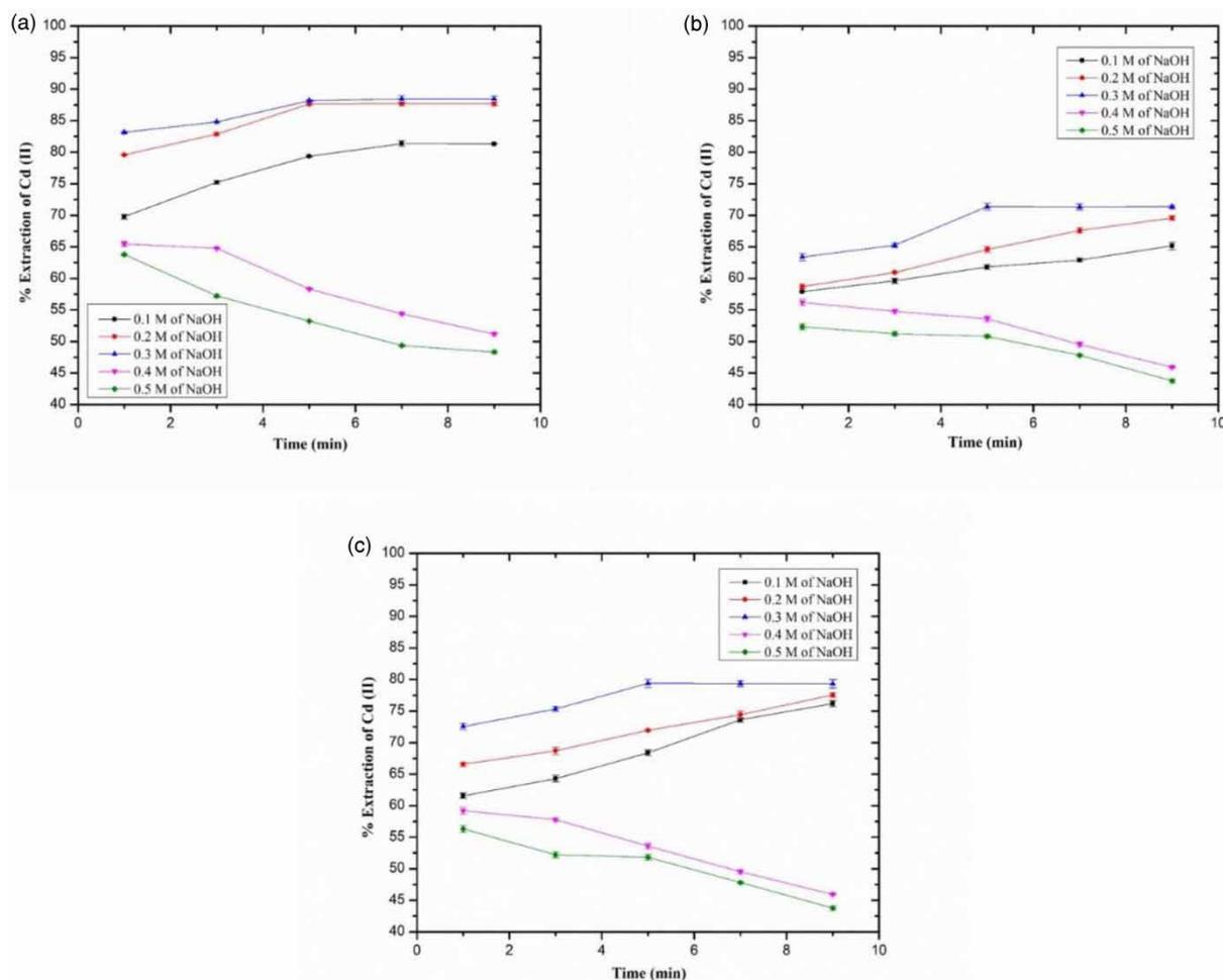
**Figure 5** | Effect of stripping phase concentration on percentage extraction of Cd (II) using various surfactants (a) ASNWs, (b) alumina and (c) SPAN 80.
