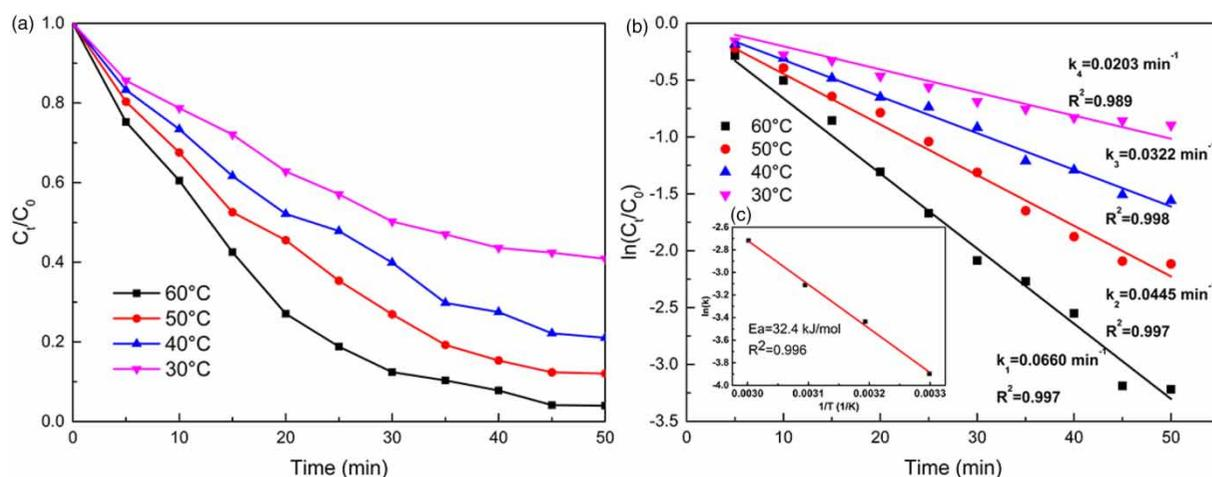
**Figure 7** | The effect of temperature on the RhB degradation and the kinetics data of the reaction. (a) The decolorization efficiency of RhB at different temperatures. (b) Plots of  $\ln(C_t/C_0)$  versus time for the RhB degradation. (c) Plots of  $\ln(k)$  versus  $(1/T)$ . (pH = 7, initial dye concentration = 400 mg/L, H $_2$ O $_2$  dosage = 40 mM, M2 dosage = 1 g/L.)
