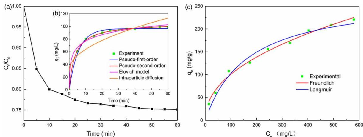
**Figure 5** | Adsorption experiment of M2. (a) Adsorption properties of RhB (400 mg/L) over M2 ( $T = 60\text{ }^{\circ}\text{C}$ ). (b) The theoretical and experimental adsorption kinetic data of RhB ( $T = 60\text{ }^{\circ}\text{C}$ ). (c) The theoretical and experimental adsorption isotherm data of RhB ( $T = 20\text{ }^{\circ}\text{C}$ ). (Reaction conditions: catalyst dosage = 1.0 g/L, pH = 7.)
