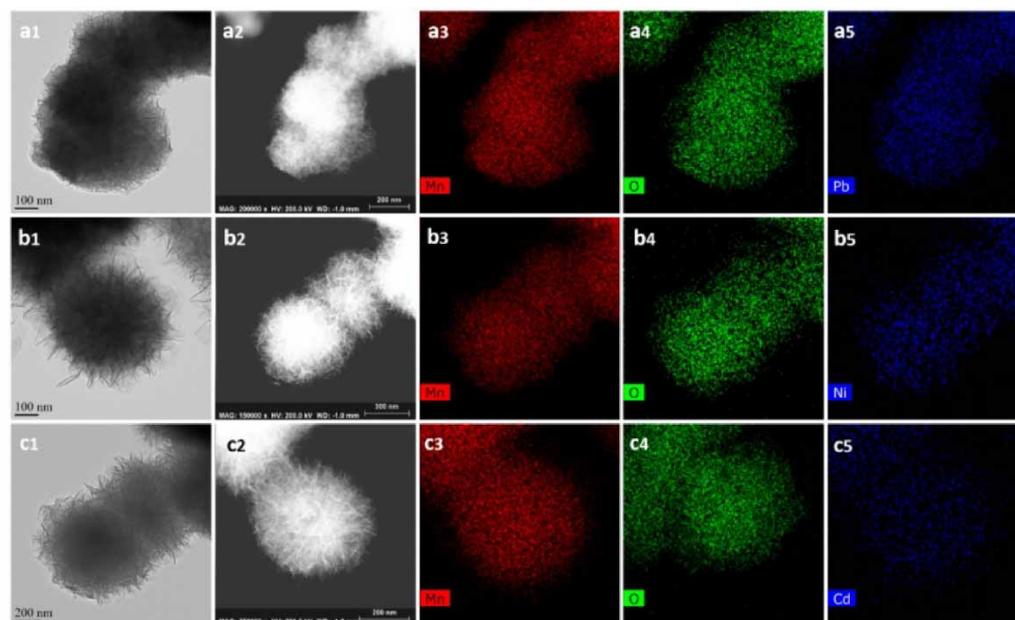
**Figure 9** | TEM image of HMO after adsorption of (a<sub>1</sub>) Pb(II), (b<sub>1</sub>) Ni(II), and (c<sub>1</sub>) Cd(II); (a<sub>2</sub>)~(c<sub>2</sub>) HAADF-STEM image of HMO after adsorption of (a<sub>2</sub>) Pb(II), (b<sub>2</sub>) Ni(II), and (c<sub>2</sub>) Cd(II); the corresponding EDS mapping of HMO after adsorption of (a<sub>3</sub>-a<sub>5</sub>) Pb(II), (b<sub>3</sub>-b<sub>5</sub>) Ni(II), and (c<sub>3</sub>-c<sub>5</sub>) Cd(II).
