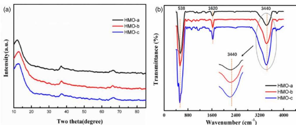
**Figure 1** | (a) The XRD spectrum of different HMO, (b) The FTIR spectrum of different HMO.
