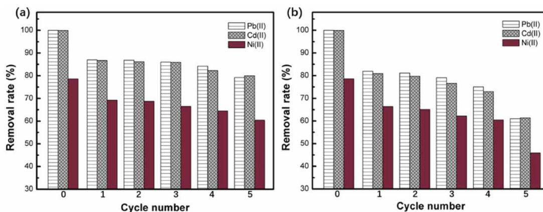
Figure 8 | Heavy metal removal rate of HMO-a in successive cycles: desorption agent (a)  $KMnO_4$ , (b) HCl.
