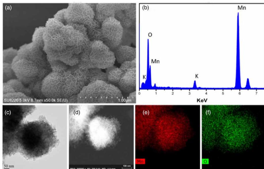
**Figure 2** | Morphologies of HMO-a: (a) SEM image of HMO-a; (b) the corresponding EDS spectrum of HMO-a; (c) TEM image of HMO-a; (d) HAADF-STEM image of HMO-a; (e,f) TEM image and the corresponding EDS mapping: Mn (red zone), O (green zone).
