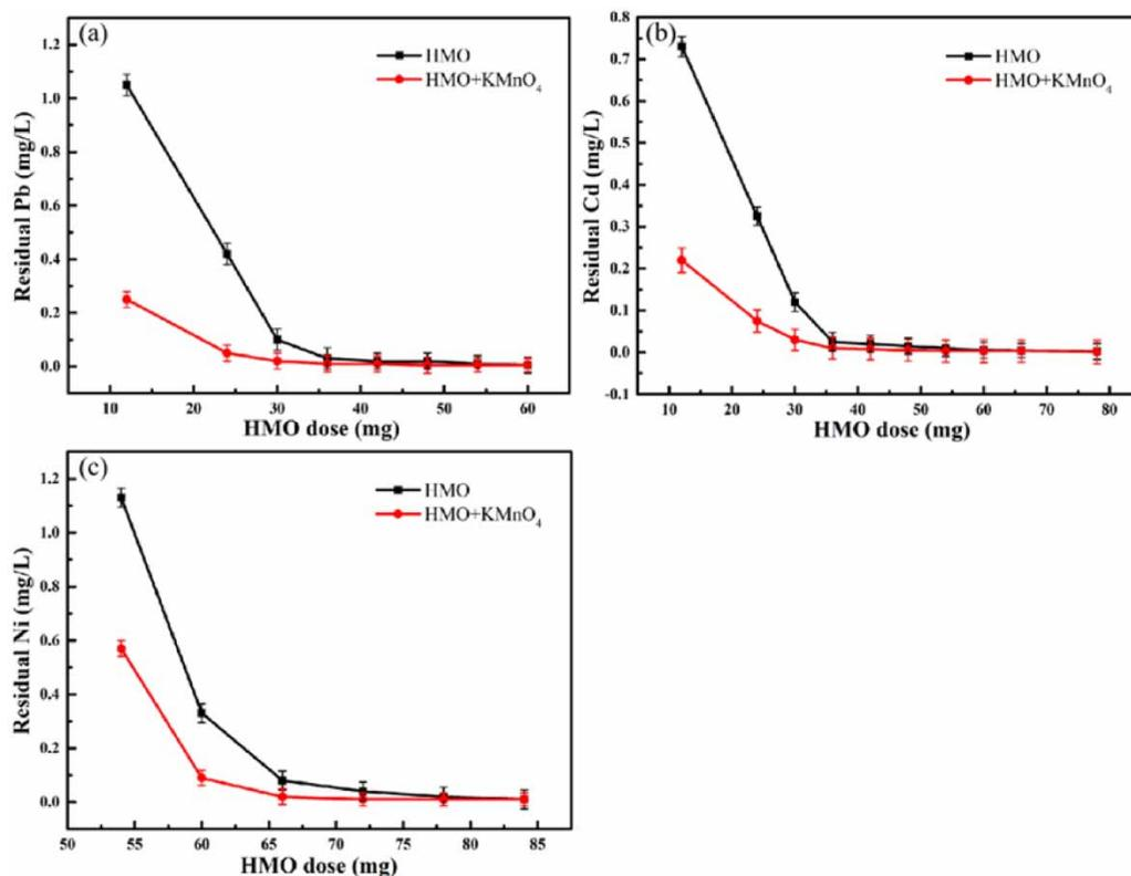
Figure 4 | The depth removal of (a) Pb (II), (b) Cd (II) and (c) Ni (II) with HMO combined with KMnO<sub>4</sub>.
