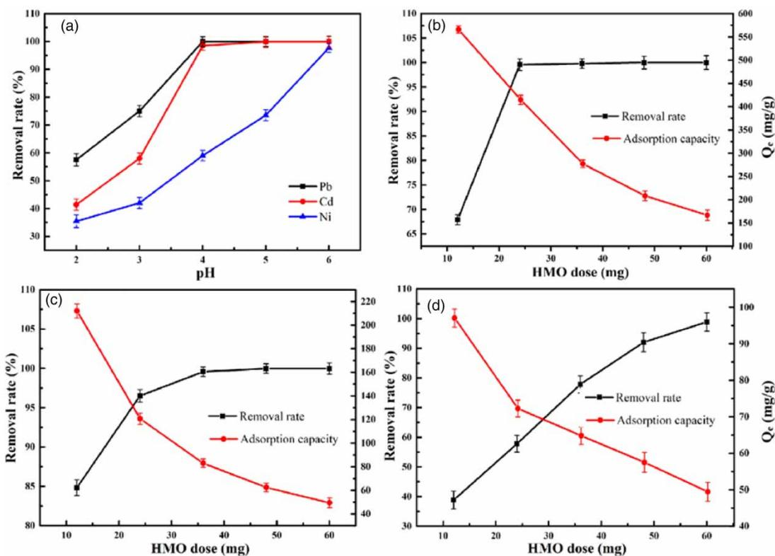
Figure 3 | (a) Effect of pH on Pb (II), Cd (II) and Ni (II) removal; effect of HMO dosage on (b) Pb (II), (c) Cd (II), and (d) Ni (II) removal.
