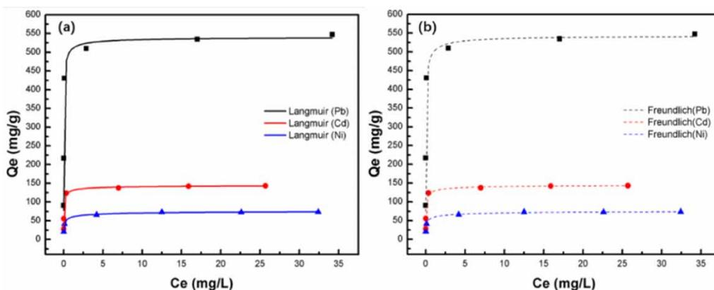
**Figure 6** | Adsorption isotherms of Pb (II), Cd (II) and Ni (II) onto HMO at pH 4.0 and 298.15 K.
