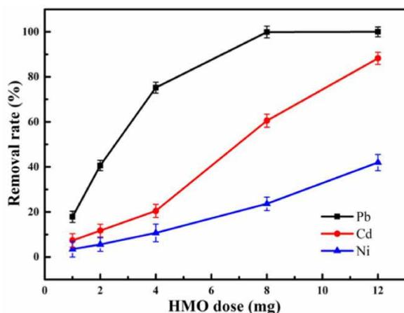
Figure 5 | Effect of co-existing heavy metal ions on heavy metal removal.
