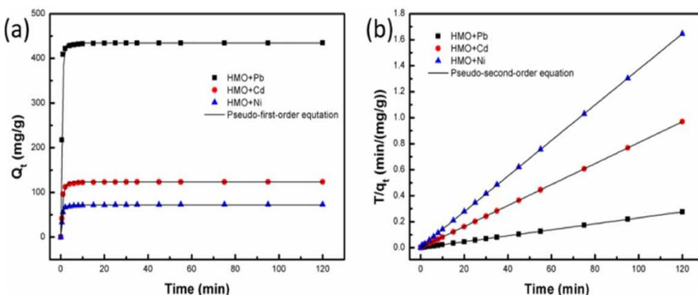
**Figure 7** | Pseudo-first-order and Pseudo-second-order of Pb (II), Cd (II) and Ni (II) adsorption onto HMO at pH 4.0 and 298.15 K.
