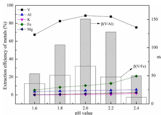
**Figure 9** | Effect of pH value on extraction and separation of vanadium and foreign ions. Experimental conditions: [extractant 7101]:[sec-octyl alcohols] = 10:10 (v/v), [extractant 7101+ sec-octyl alcohols]/[Sulphonated kerosene] = 20:80 (v/v), O/A = 1:1, time = 4 min, stirring speed = 40 r/min.
