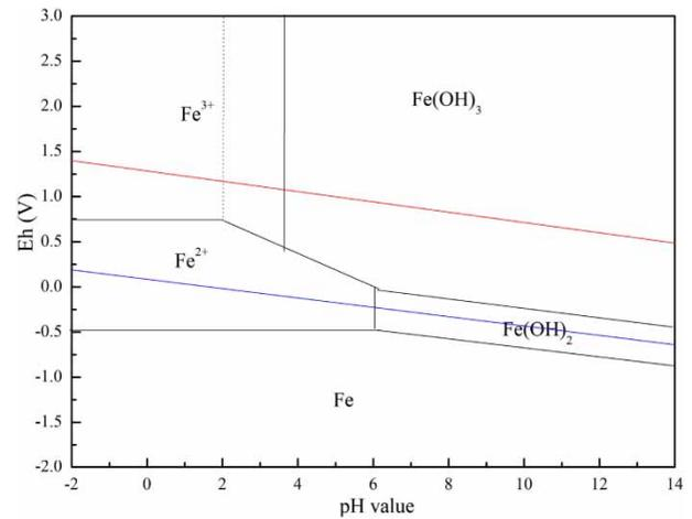
Figure 4 | Thermodynamics diagram for the iron solution.
