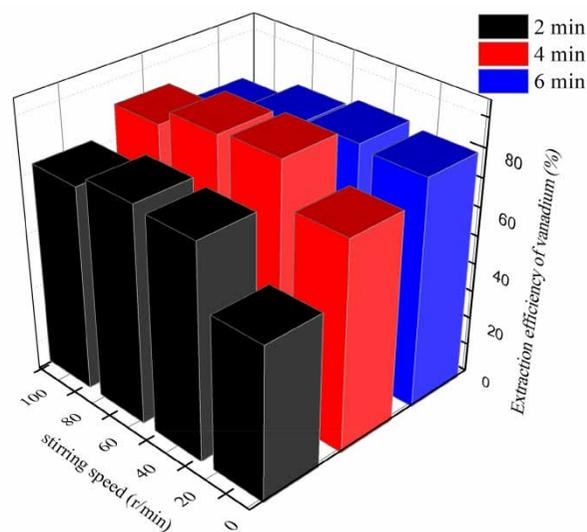
**Figure 10** | Effect of stirring speed and time on extraction of vanadium. Experimental conditions: [extractant 7101]:[sec-octyl alcohols] = 10:10 (v/v), [extractant 7101+ sec-octyl alcohols]/[Sulphonated kerosene] = 20:80 (v/v), O/A = 1:1, pH = 2.0  $\pm$  0.05.
