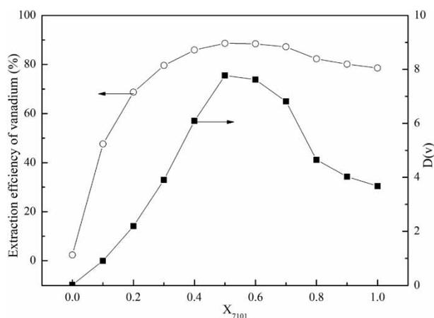
**Figure 7** | Extraction of vanadium with a mixture of extractant 7101 and sec-octyl alcohols. Experimental conditions:  $\text{pH} = 2.0 \pm 0.05$ ,  $O/A = 1:1$ , [extractant 7101+sec-octyl alcohols]/[Sulphonated kerosene] = 20:80 (v/v), time = 4 min, stirring speed = 40 r/min.
