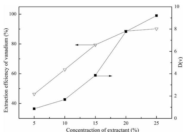
**Figure 8** | Effect of extractant concentration on recovery of vanadium with extractant 7101 and sec-octyl alcohols. Experimental conditions:  $\text{pH} = 2.0 \pm 0.05$ , [extractant 7101]:[sec-octyl alcohols] = 10:10 (v/v),  $O/A = 1:1$ , time = 4 min, stirring speed = 40 r/min.
