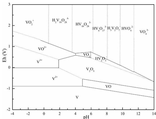
Figure 12 | Eh-pH diagram of vanadium in the solution.
