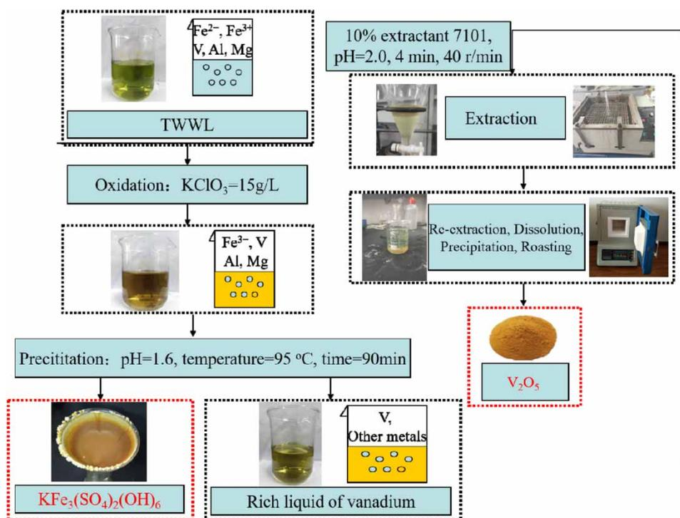
Figure 15 | Flow sheet of separation of iron and vanadium from TWWL.
