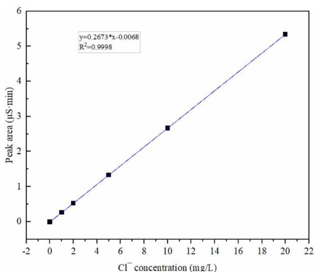
Figure 1 | Standard curve of chloride ions.
