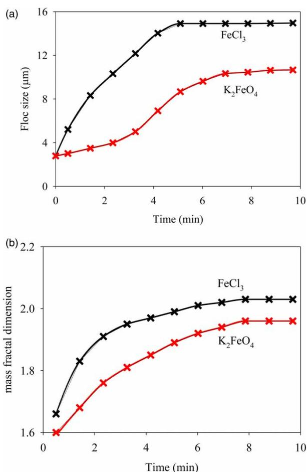
**Figure 2** | Experimental and simulated kaolin coagulation induced by  $K_2FeO_4$  and  $FeCl_3$ . (a) coagulation kinetics; (b) mass fractal dimension. Experimental conditions: dosage of Fe(VI) and  $FeCl_3 = 150 \mu M$ ,  $pH = 7$ ; shear rate =  $50 s^{-1}$ ; temperature =  $25^\circ C$ . Notes: the data point is the experimental results whereas the connecting line shows the simulation result.
