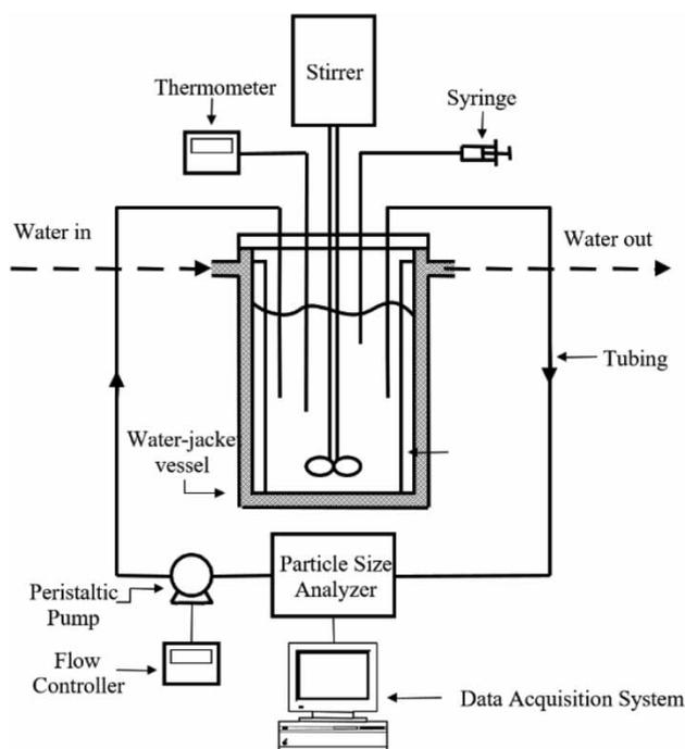
Figure 1 | Schematic of kaolin coagulation setup.
