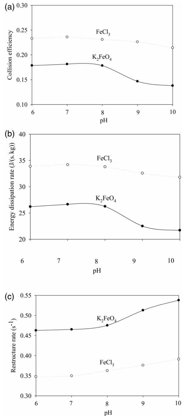
**Figure 6** | Effect of pH on (a) collision efficiency, (b) energy dissipation rate and (c) restructure rate. Experimental conditions: dosage of ferrate(VI) and  $\text{FeCl}_3 = 150 \mu\text{M}$ ; shear rate =  $50 \text{ s}^{-1}$ ; temperature =  $25^\circ\text{C}$ .
