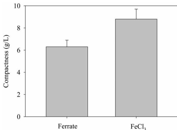
**Figure 7** | Ratio of the mass to volume of settled kaolin flocs (compactness). Experimental conditions: dosage of ferrate(VI) and FeCl<sub>3</sub> = 150 μM; pH = 7; shear rate = 50 s<sup>-1</sup>; temperature = 25 °C.
