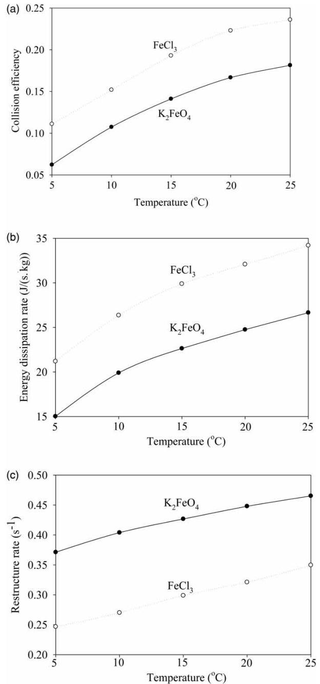
**Figure 5** | Effect of temperature on (a) collision efficiency, (b) energy dissipation rate and (c) restructure rate. Experimental conditions: dosage of ferrate(VI) and FeCl<sub>3</sub> = 150 μM; pH = 7; shear rate = 50 s<sup>-1</sup>.
