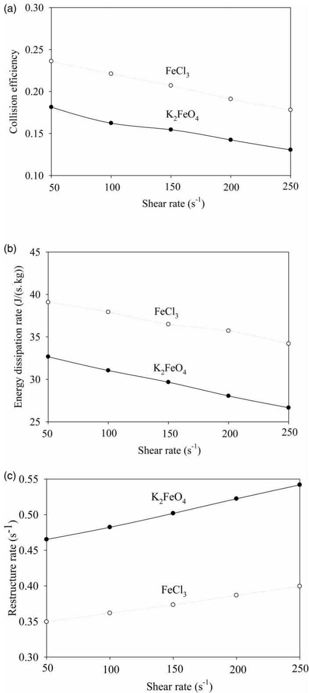
**Figure 4** | Effect of shear rate on (a) collision efficiency, (b) energy dissipation rate and (c) restructure rate. Experimental conditions: dosage of ferrate(VI) and FeCl<sub>3</sub> = 150 μM; pH = 7; temperature = 25 °C.
