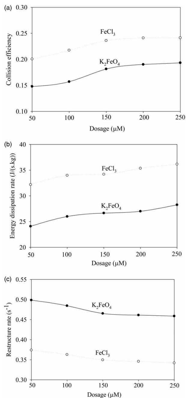
**Figure 3** | Potassium ferrate(VI) and FeCl<sub>3</sub> dosage effect on (a) collision efficiency, (b) energy dissipation rate and (c) restructure rate. Experimental conditions: pH = 7; shear rate = 50 s<sup>-1</sup>; temperature = 25 °C.
