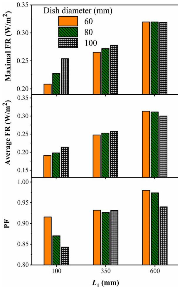
**Figure 2** | Simulated FR and PF values on target surfaces induced by single-aperture constrained beams with different distances ( $L_1$ ) from the UV lamp to the aperture (collimator diameter = 100 mm, and distance between lamp and Petri dish = 900 mm).
