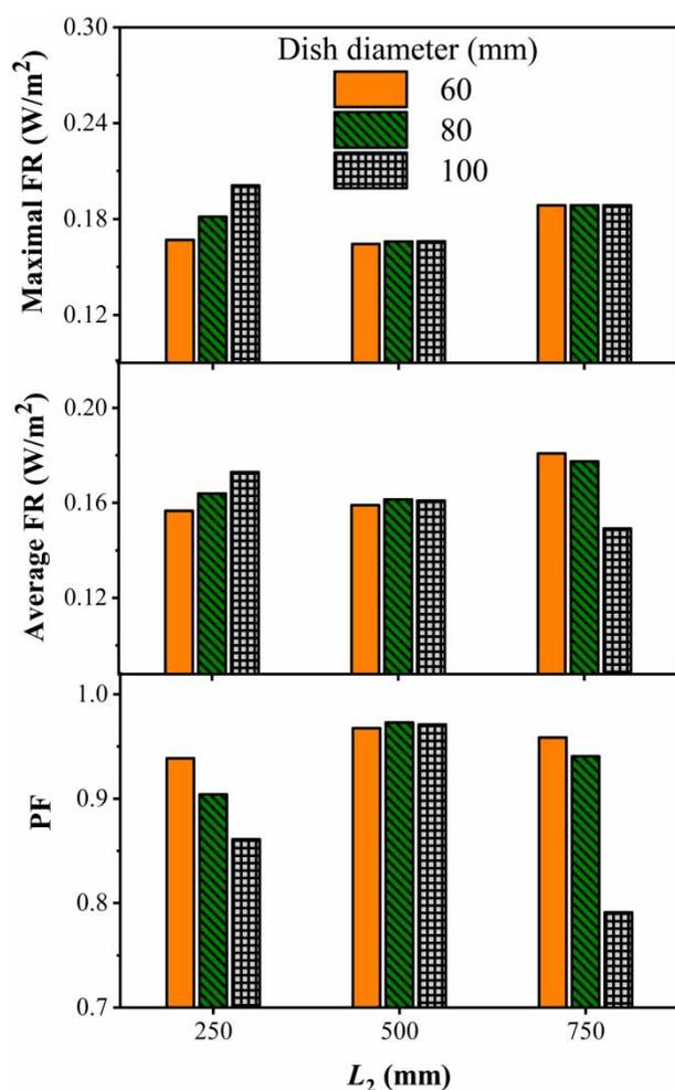
**Figure 5** | Simulated FR and PF values on target surfaces in two-aperture QCBA with different distances ( $L_2$ ) between apertures (collimator diameter = 100 mm, distance between lamp and Petri dish = 900 mm, distance between lamp and upper aperture = 100 mm).
