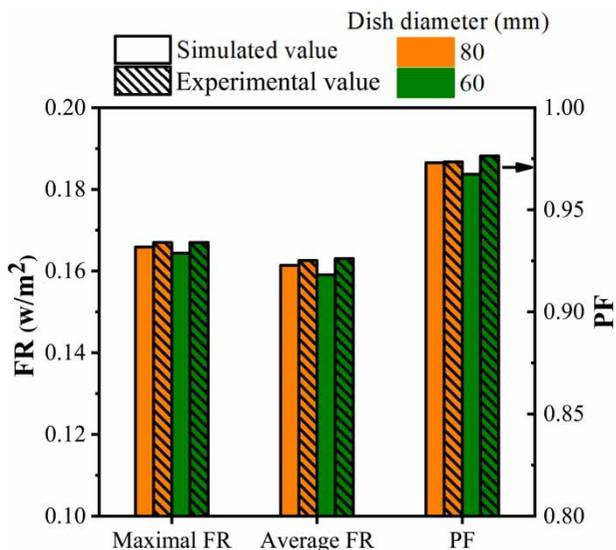
**Figure 7** | Comparison of the experimental and simulated FR distribution in the constructed QCBA (two successive apertures, with a BOS-1T5 UVC lamp; collimator diameter = 100 mm, distances from the UV lamp to the upper aperture = 100 mm, distance between each aperture = 500 mm, and distance between lamp and Petri dish = 900 mm).
