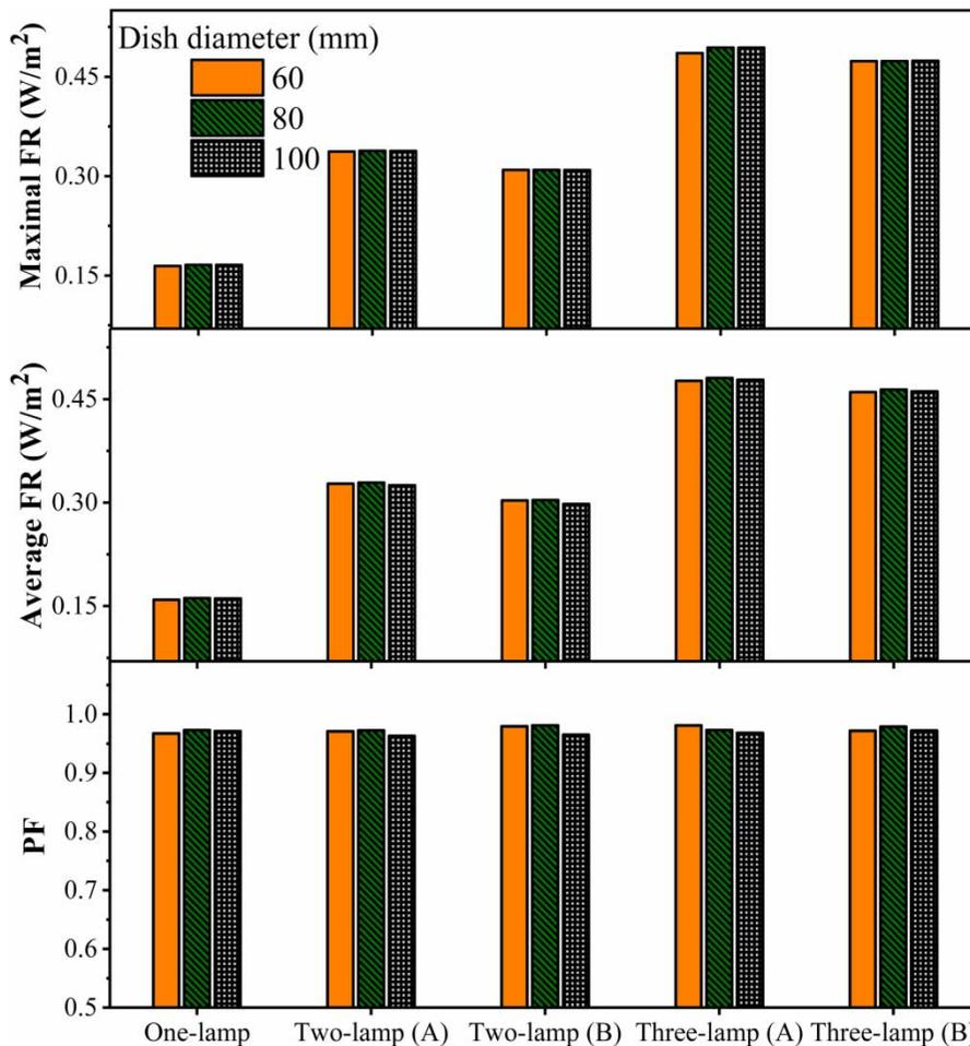
**Figure 6** | Simulated FR and PF values on target surfaces in two-aperture QCBA with different lamp number. (A) pattern with lamps adjacent in the middle over the collimator hole; (B) pattern of lamps evenly arranged along the diameter of the target area (collimator diameter = 100 mm, distance between lamp and Petri dish = 900 mm, distance between each aperture = 500 mm, distance between lamp and upper aperture = 100 mm).
