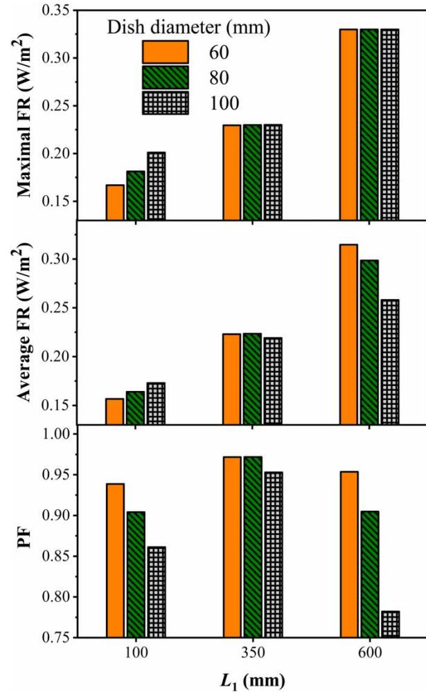
**Figure 4** | Simulated FR and PF values on target surfaces in two-aperture-type QCBA with different distances ( $L_1$ ) from the UV lamp to the upper aperture (collimator diameter = 100 mm, distance between lamp and Petri dish = 900 mm, distance between each aperture = 250 mm).
