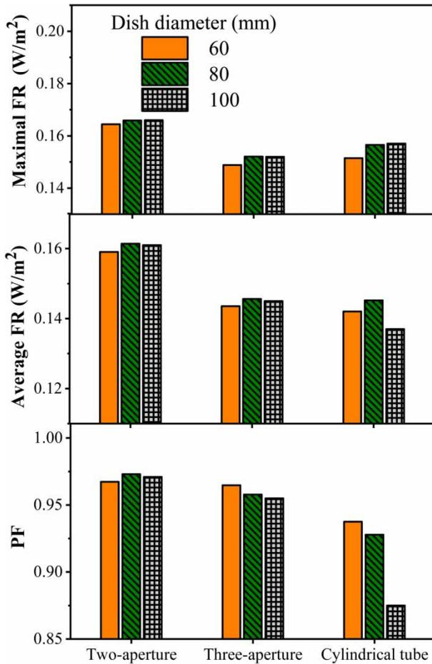
**Figure 3** | Simulated FR and PF values on target surfaces induced by multiple successive apertures and cylindrical tube (collimator diameter = 100 mm, distance between lamp and Petri dish = 900 mm, length of collimator = 500 mm, distance between lamp and upper aperture = 100 mm).
