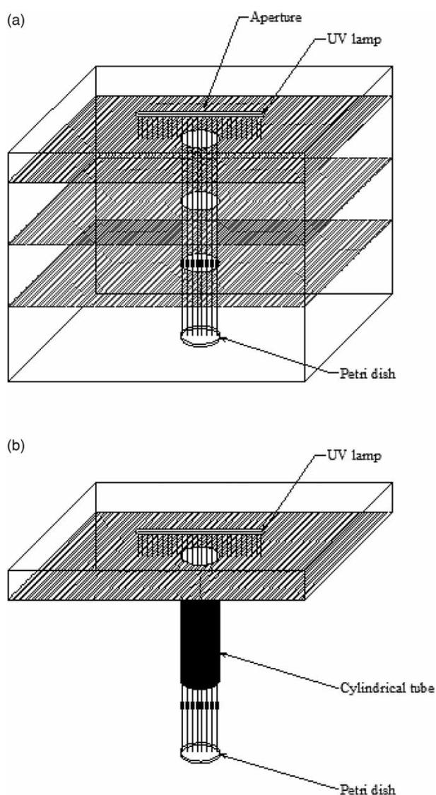
**Figure 1** | Schematic diagram of two modelled QCBA: (a) successive apertures type, and (b) cylindrical tube type.
