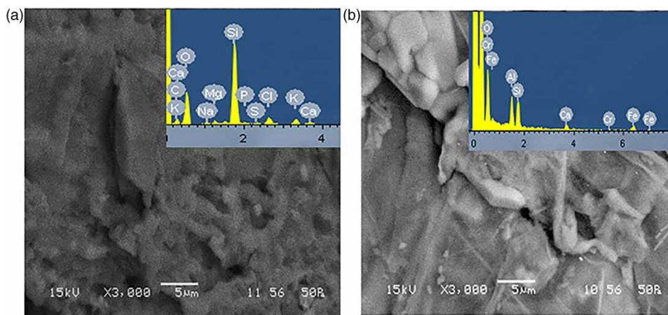
**Figure 2** | SEM-EDX images of the activated charcoal (a) without (control) and (b) with (10 mg/L) chromium ions after treated 15 cm of bed height.
