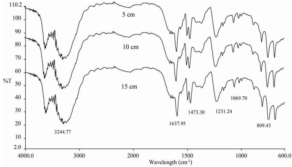
**Figure 3** | FTIR spectra of the activated charcoal with different bed height a constant initial concentration 10 mg/L of chromium solutions at pH 7.
