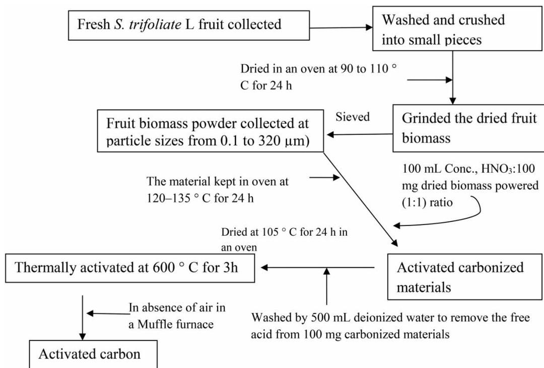
Figure 1 | Preparation procedure flow chart of activated charcoal derived from *S. trifoliata* L fruit biomass.
