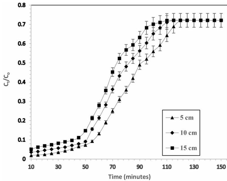
**Figure 4** | Effect of bed height on the removal of Cr(VI) in the fixed bed column (Initial concentration: 10 mg/L; flow rate: 0.5 mL/min; pH: 7 and temperature: 30 °C).
