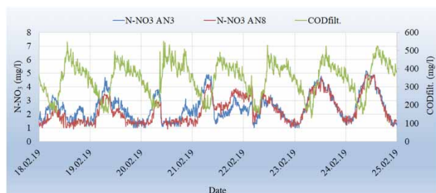
Figure 8 | N-NO 3 concentration in the outlet of aeration basin depending on chemical oxygen demand in filtrate (COD fit ).
