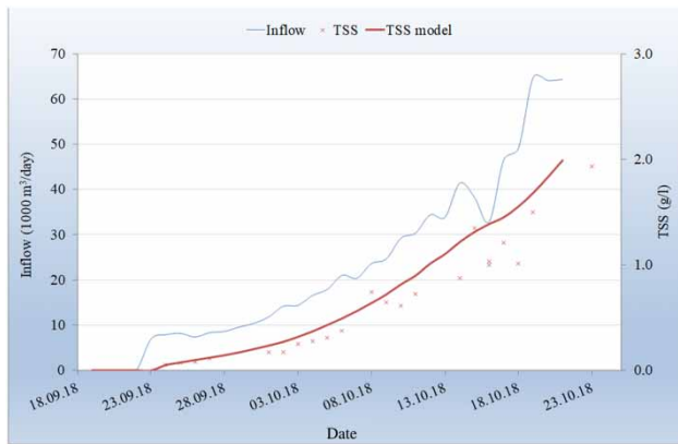
Figure 3 | Treated water volume and TSS concentration of activated sludge – NWL.
