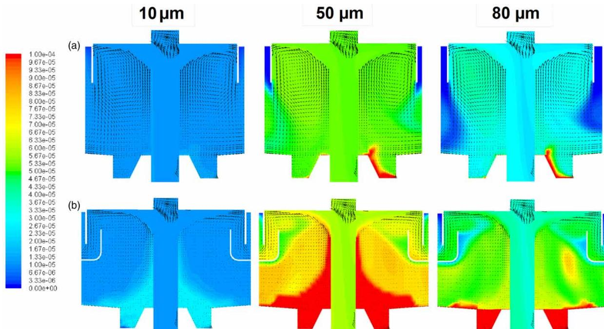
**Figure 7** | Solid volume fraction in inlet zone and sludge hopper (a) OPST and (b) NPST. Note: The solids concentration can be obtained by multiplying the solids volume fraction by the density of the solids ( $1,396.5 \text{ kg/m}^3$ ).
