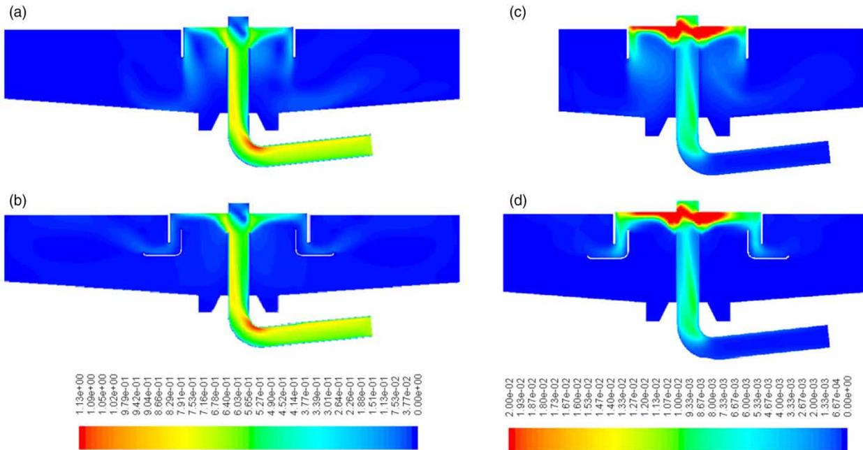
**Figure 6** | Velocity contours (m/s) (a) OPST and (b) NPST and contour of turbulence kinetic energy ( $\text{m}^2/\text{s}^2$ ) (c) OPST and (d) NPST.
