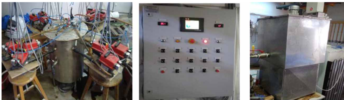
Figure 8 | The experimental setup: PABR, programmable logic computer (PLC) and feedstocks storage tank.
