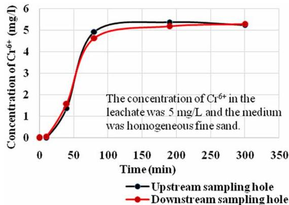
**Figure 6** | Two-dimensional migration of Cr<sup>6+</sup> in homogeneous sand media.
