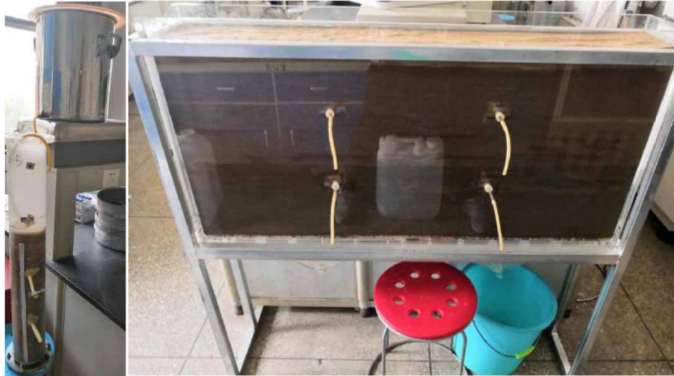
Figure 3 | Infiltration experimental apparatus (left: cylindrical, one-dimensional, vertical infiltration column; right: box-shaped, two-dimensional infiltration tank).
