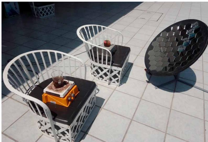
**Figure 8** | Image of the experimentation of the photo-Fenton tests under direct sunlight and using the solar parabolic concentrator. Please refer to the online version of this paper to see this figure in colour: <http://dx.doi.org/10.2166/wst.2021.438>.
