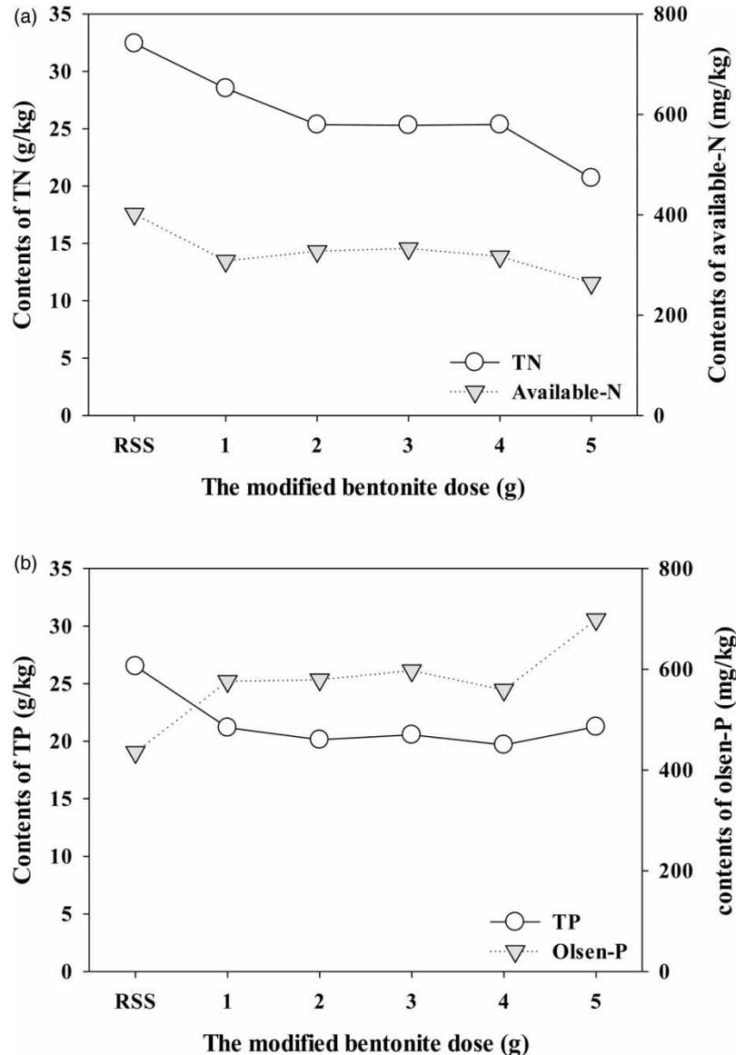
**Figure 3** | The retention of nutrients in the sewage sludge (weight of each sample = 50 g) as a function of the modified bentonite dose (1–5 g): (a) nitrogen species and (b) phosphorus species (RSS: raw sewage sludge).
