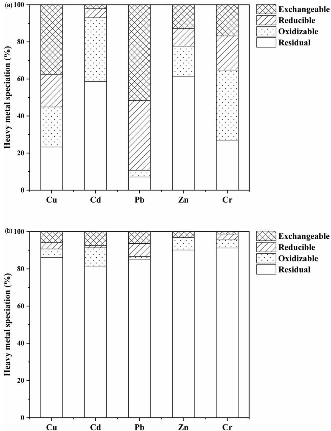
**Figure 2** | Comparison of the heavy metal speciation in the sewage sludge (weight of each sample = 50 g) before and after conditioning with 3 g of the modified bentonite: (a) the raw sewage sludge and (b) the conditioned sewage sludge.
