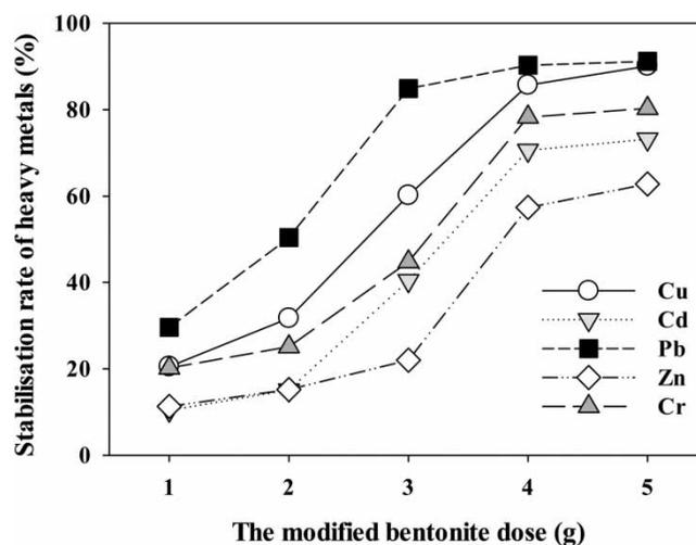
**Figure 1** | Stabilization rate of the heavy metals from the sewage sludge (weight of each sample = 50 g) as a function of the modified bentonite dose (1–5 g).
