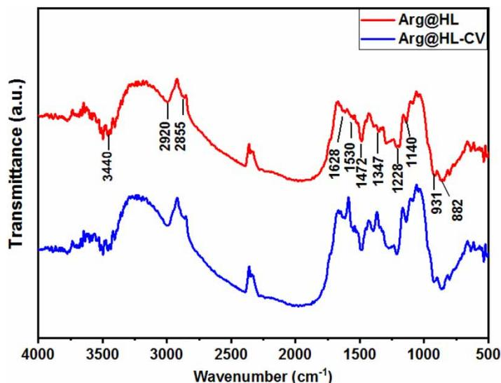
**Figure 3** | FTIR spectrums of Arg-heliotrope leaves (Arg@HL) and CV loaded Arg-heliotrope leaves (Arg@HL-CV).
