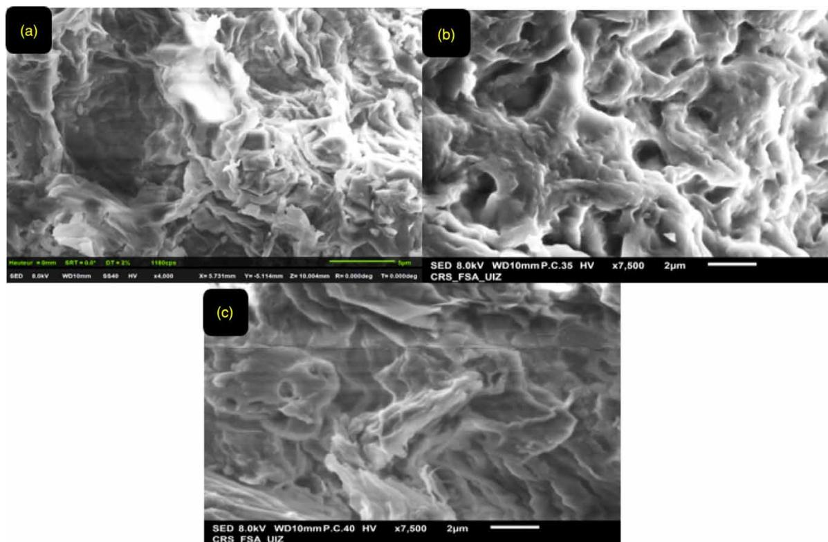
**Figure 2** | SEM images of (a) the raw used heliotrope leaves. Arginine-modified heliotrope leaves (Arg@HL) (b) before and (c) after CV adsorption (Arg@HL-CV).
