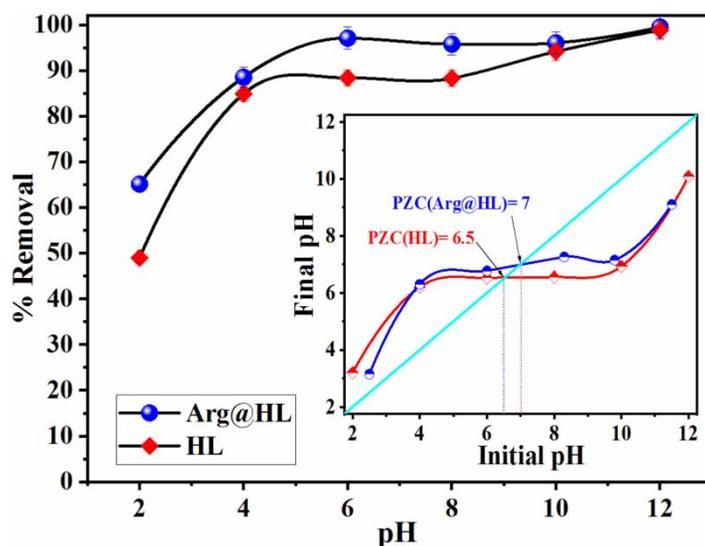
**Figure 6** | pH influence on the efficiency of CV dye adsorption in the presence of HL and Arg@HL ( $C_0 = 20 \text{ mg}\cdot\text{L}^{-1}$ , time of adsorption = 240 min, adsorbent amount = 0.75 g/L and  $T = 298 \text{ K}$ ). The inset is the PZC of HL and Arg@HL.
