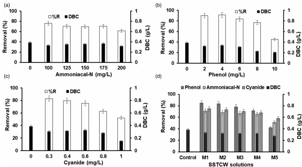
**Figure 2** | (a) TLS of consortium in simulated ammoniacal-N solutions, (b) TLS of consortium in simulated phenol solutions, (c) TLS of consortium in simulated cyanide solutions, (d) TLS of consortium in SSTCW solutions.
