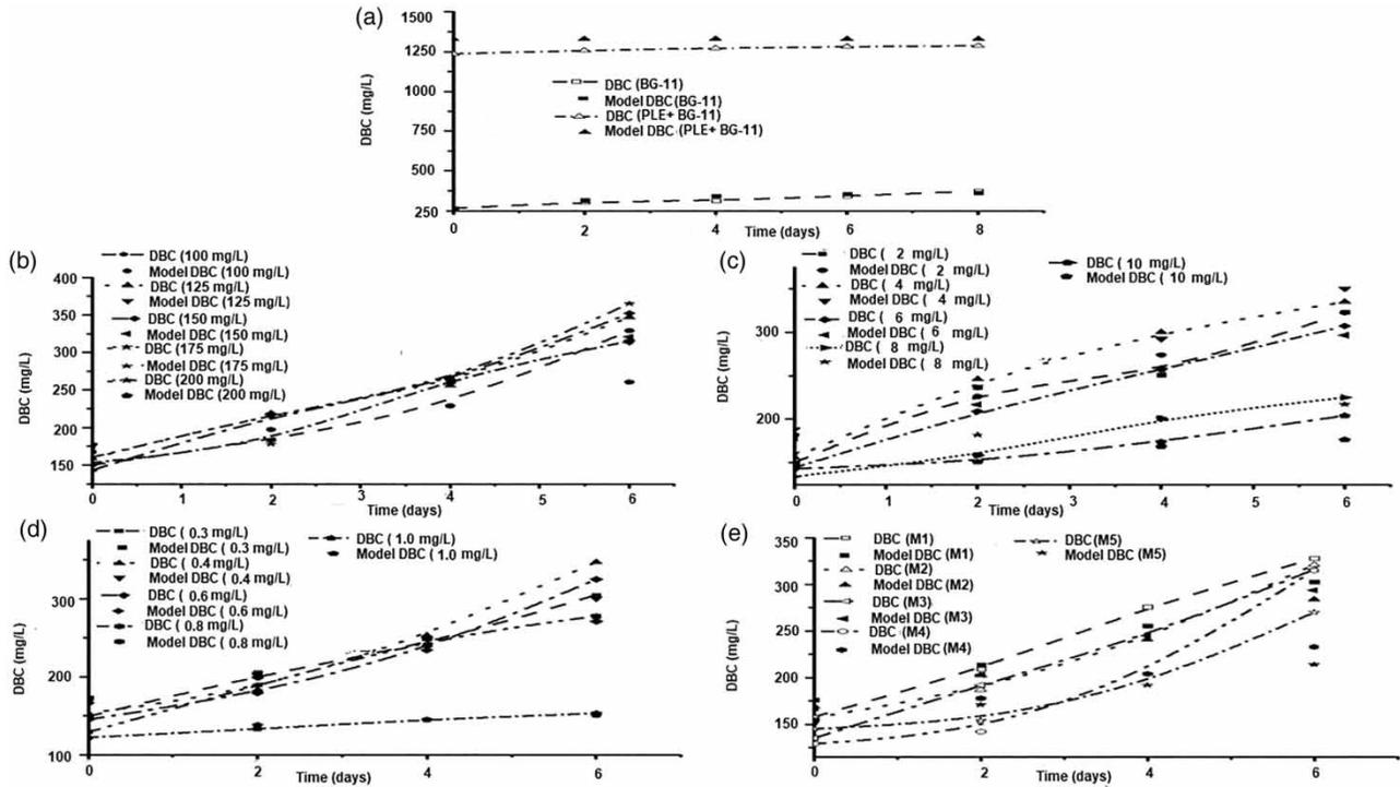
**Figure 5** | Comparison of experimental and model-predicted DBC during exponential phase at different systems: (a) in different media (BG-11 and PLE-enriched BG-11 media), (b) in simulated solutions of  $\text{NH}_4^+$ , (c) in simulated solutions of phenol, (d) in simulated solutions of cyanide and (e) in SSTCW solutions.
