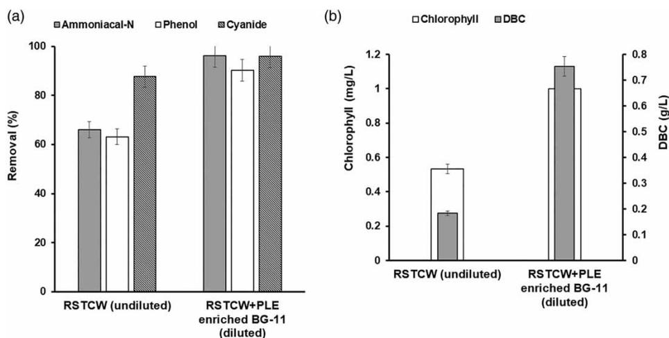
**Figure 4** | (a) Bioremoval of  $\text{NH}_4^+$  (ammoniacal-N), phenol and cyanide using a consortium of *Synechococcus* sp. and *Chlorella* sp. from RSTCW and (b) production of DBC and chlorophyll content during the treatment of RSTCW.
