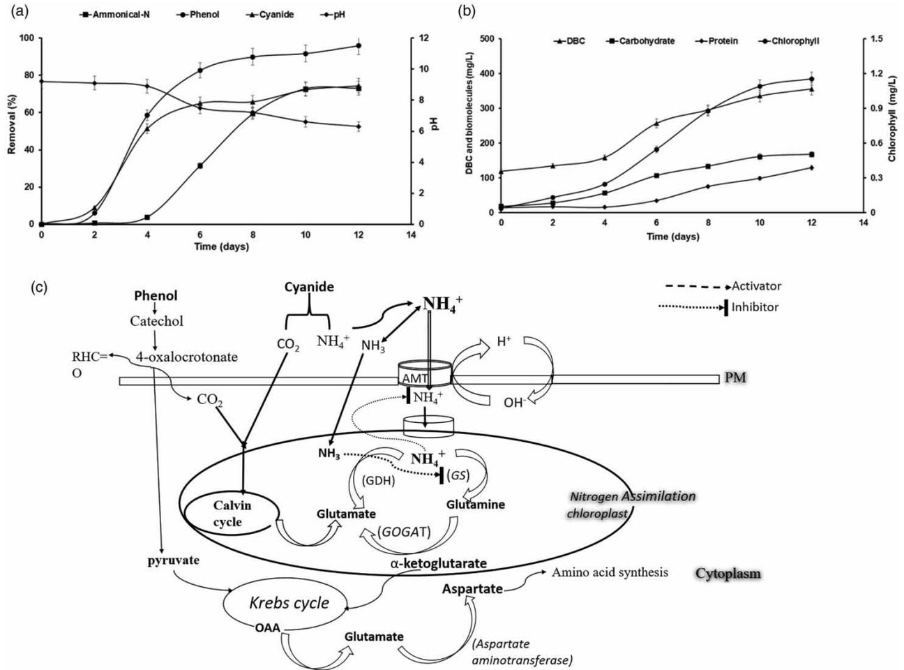
**Figure 3** | Time variation studies on: (a) the removal of pollutants from SSTCW solution (M4) and variation of pH of the SSTCW and (b) the production of biomass and biomolecules during treatment of SSTCW solution (M4). (c) Proposed pathways for pollutants removal from SSTCW (Gurbuz *et al.* 2004; Wang *et al.* 2019; Rai *et al.* 2020).
