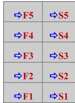
Figure 2 | Sampling zones within the WPWS PRB (F: first half area, S: second half area, ⇒flow direction).
