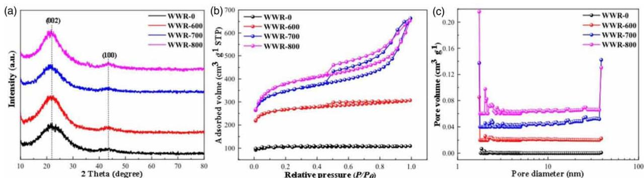
Figure 2 | (a) XRD patterns; (b) N<sub>2</sub> adsorption-desorption isotherm; (c) pore size distribution of WWR-800.
