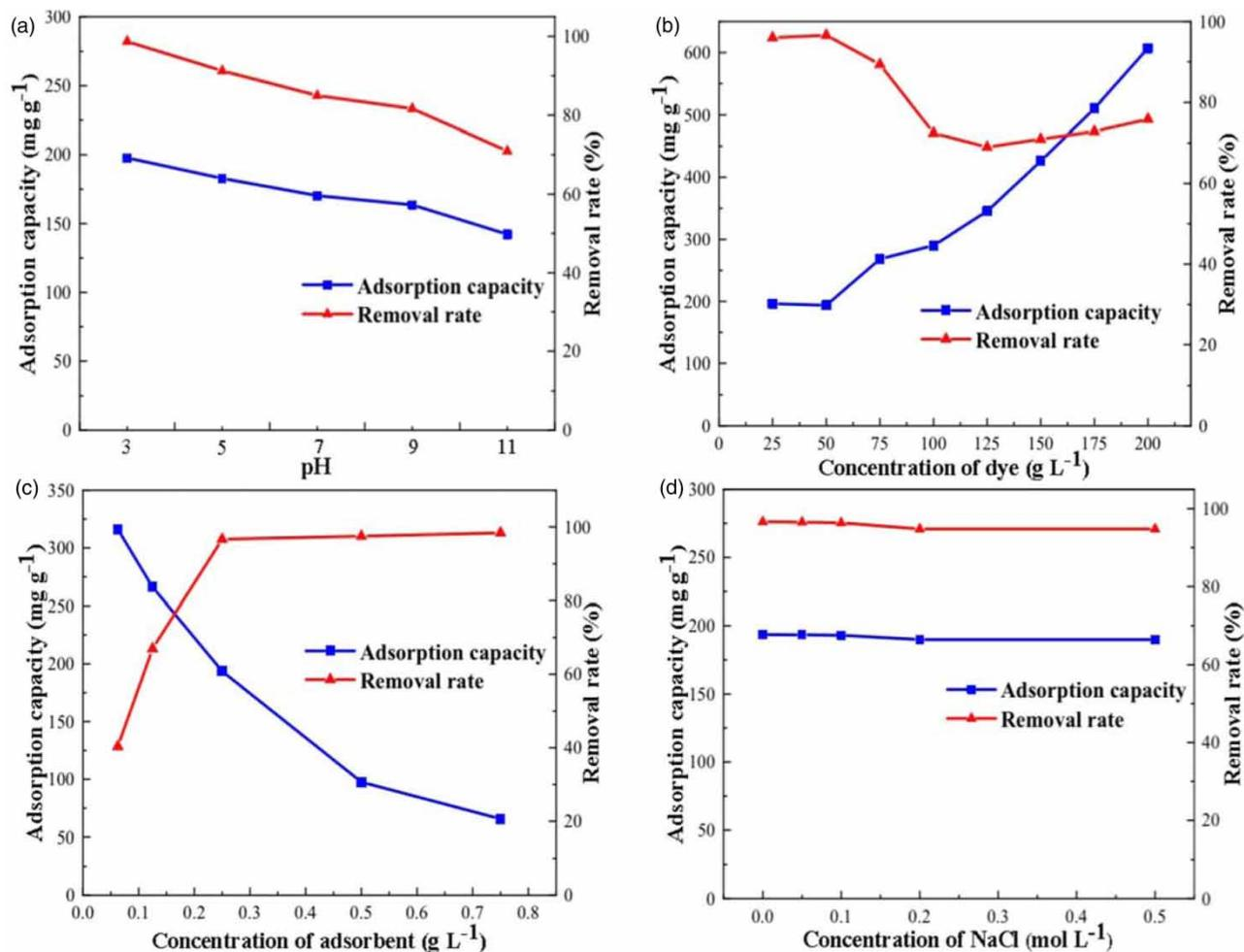
**Figure 5** | (a) Influence of different pH. 50 mg/L of MO, 12.5 mg (0.25 g/L) of WWR-800, 25 °C; (b) influence of different concentrations of MO. Condition: 12.5 mg (0.25 g/L) of WWR-800, pH = 3, 25 °C; (c) influence of different dosing of WWR-800. Condition: 50 mg/L of MO, pH = 3, 25 °C; (d) influence of different ionic strengths. Condition: 50 mg/L of MO, 12.5 mg (0.25 g/L) of WWR-800, pH = 3, 25 °C.
