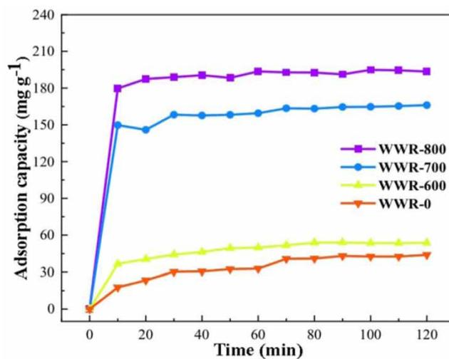
**Figure 4** | Adsorption performance of WWRs: 50 mg/L of MO, 12.5 mg (0.25 g/L) of WWRs, 25 °C.
