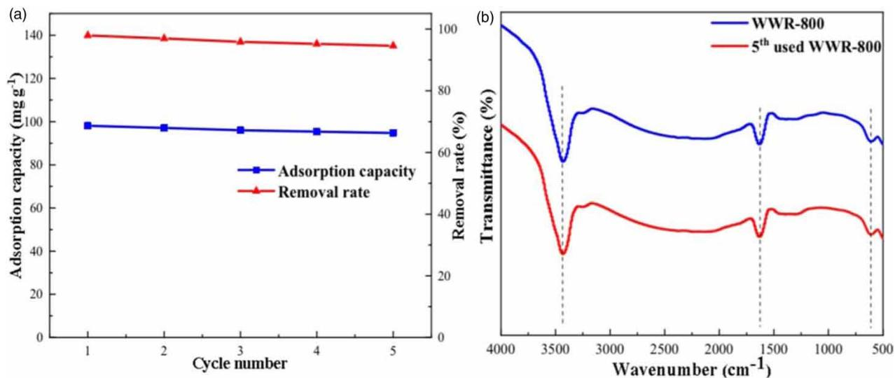
**Figure 7** | (a) Adsorption of MO using the recycled adsorbent WWR-800; (b) FT-IR of the 5th used WWR-800. Condition: 50 mg/L of MO, 20 mg (0.5 g/L) of WWR-800, 25 °C.
