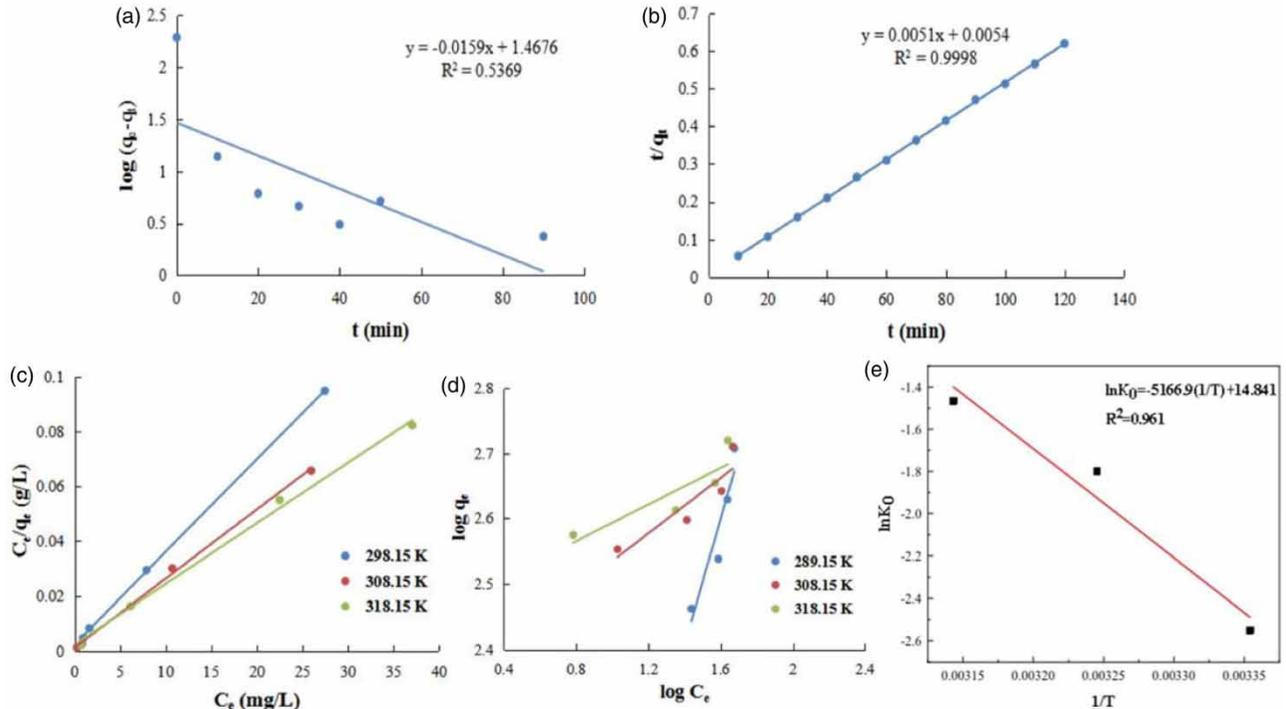
**Figure 6** | (a) Pseudo-first order kinetic models fitting of MO by WWR-800; (b) pseudo-second order kinetic models fitting of MO by WWR-800; (c) Langmuir adsorption isotherms for adsorption of MO on WWR-800; (d) Freundlich adsorption isotherms for adsorption of MO on WWR-800 (e) Vant Hoff's plot for MO adsorption by WWR-800.
