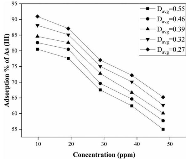
**Figure 5** | Impact of particle size on adsorption of As(III) at constant bed height (10 cm) and constant pH of the solution (pH 6).
