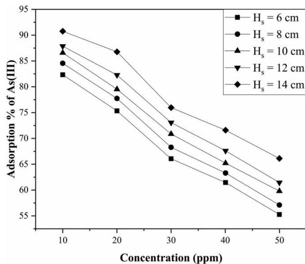
**Figure 6** | Impact of static bed height on adsorption of As(III) at constant particle size (0.39 mm) and constant pH of the solution (pH 6).
