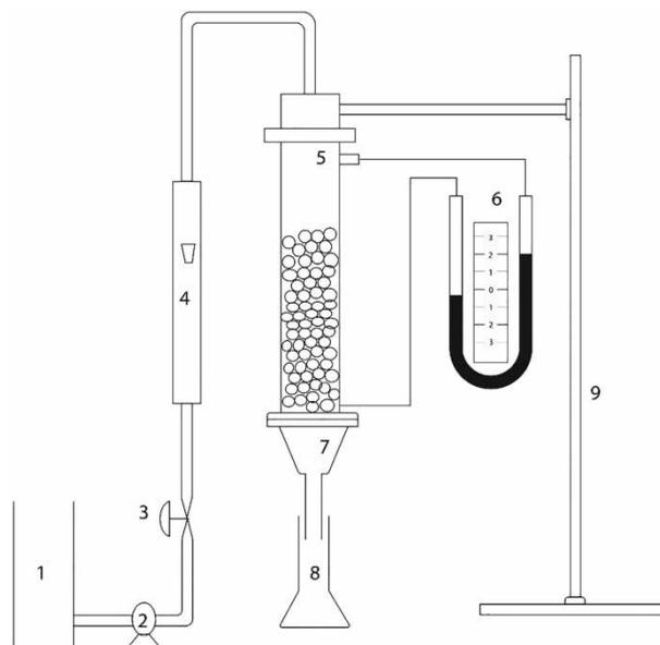
**Figure 1** | Schematic of the experimental setup: 1, liquid tank; 2, water pump; 3, control valve; 4, rotameter; 5, column bed with adsorbent; 6, u-tube manometer; 7, mesh with conical base; 8, conical vessel; 9, iron stand.
