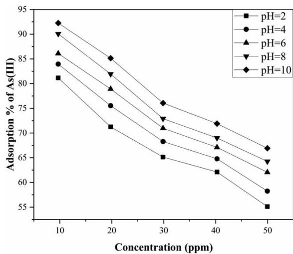
**Figure 4** | Impact of pH on adsorption of As(III) at constant bed height (10 cm) and constant average particles size (0.39 mm).
