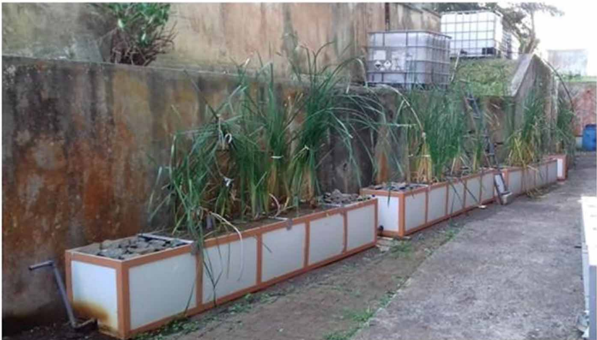
Figure 1 | Intensified and conventional experimental HSSF CWs.
